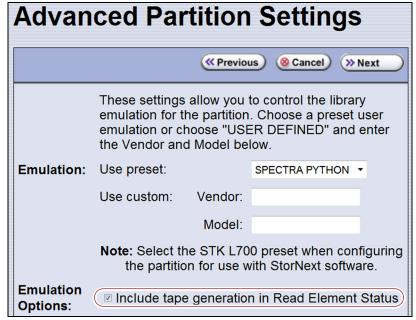
**Figure 1** Enable including media and drive generation information in the Read Element Status on the BlueScale Advanced Partition Settings screen.
