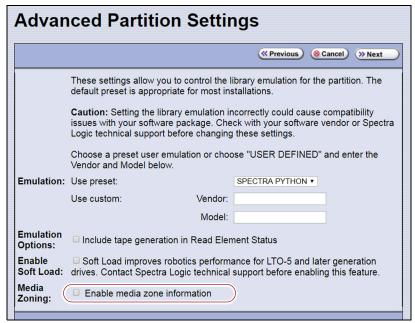
**Figure 2** Use the BlueScale Advanced Partition Settings screen to enable including zone information and TeraPack barcodes in the Read Element Status.
