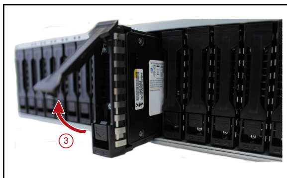
Figure 8 Remove the drive sled with drive blank and insert the drive sled with drive.
