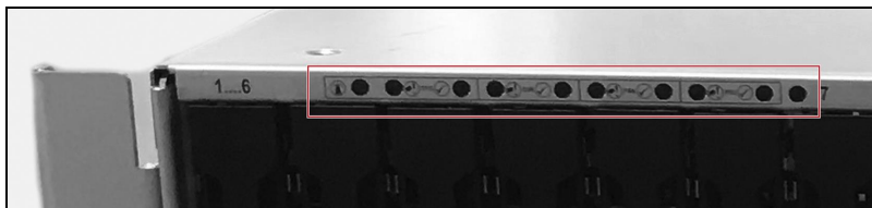
Figure 139 The top left section of the front of the Gen2 X chassis (front bezel removed) showing system status LEDs.
