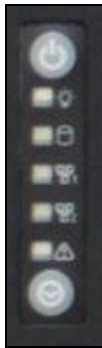
Figure 140 The top right section of the front of the Gen2 S Series chassis, with the front bezel removed, showing system status LEDs.
