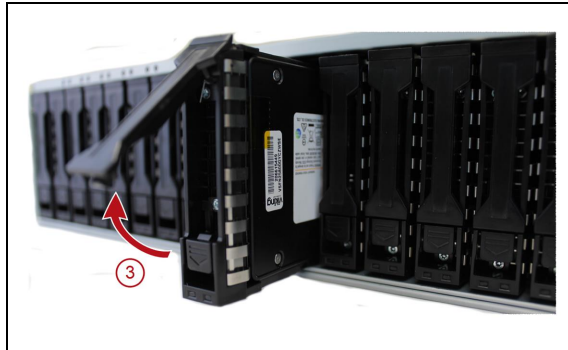
Figure 200 Remove the drive sled with drive blank and insert the drive sled with drive.
