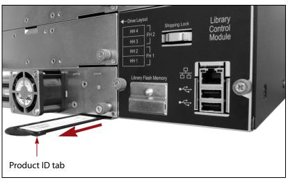
Figure 69 Slide the product ID tab out from the bottom of the library to view the library's serial number.
