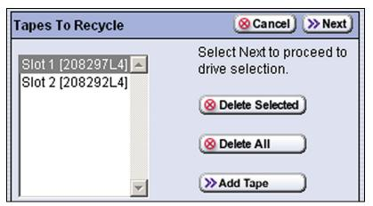
**Figure 228** The Tapes to Recycle screen.
