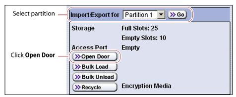
Figure 317 Select the partition and then click Open Door to open the access port.
