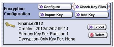
**Figure 216** Use **Check Key Files** to confirm successful export.
