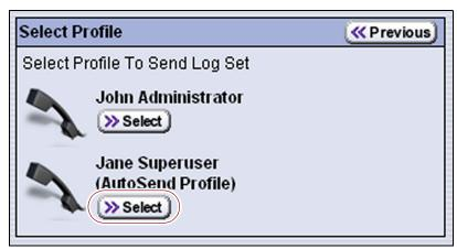
**Figure 245** Click **Select** under the profile you want to use for sending the AutoSupport ticket.
