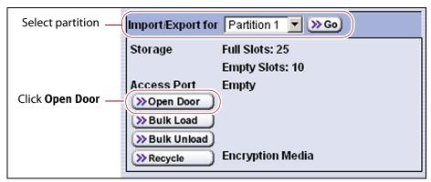
**Figure 145** Select the partition and then click **Open Door** to open the access port.
