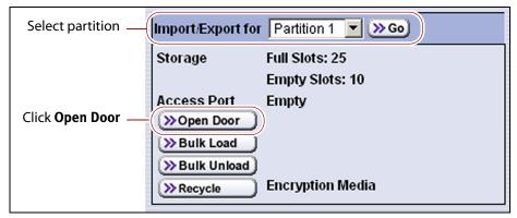
**Figure 140** Select the partition and then click **Open Door** to open the access port.
