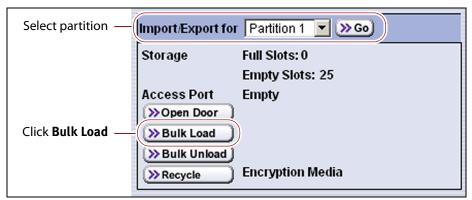
Figure 135 Select the partition and then click Bulk Load.
