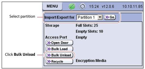
Figure 147 Select the partition and then click Bulk Unload.
