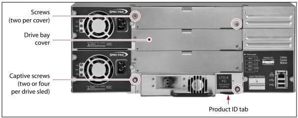
Figure 16 Loosen the captive screws securing the drive bay cover to the library.
