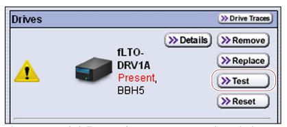
**Figure 286** Click **Test** on the Drives screen to launch the wizard.
