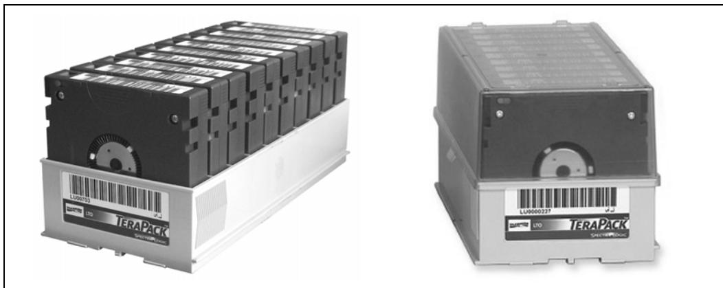
Figure 318 TeraPack magazines with barcode labeled cartridges and plastic dust cover (LTO magazines shown).
