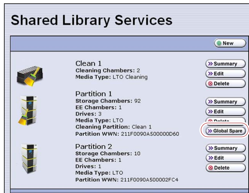
Figure 254 Click Global Spare to begin the process of replacing a partition drive with a Global Spare drive.
