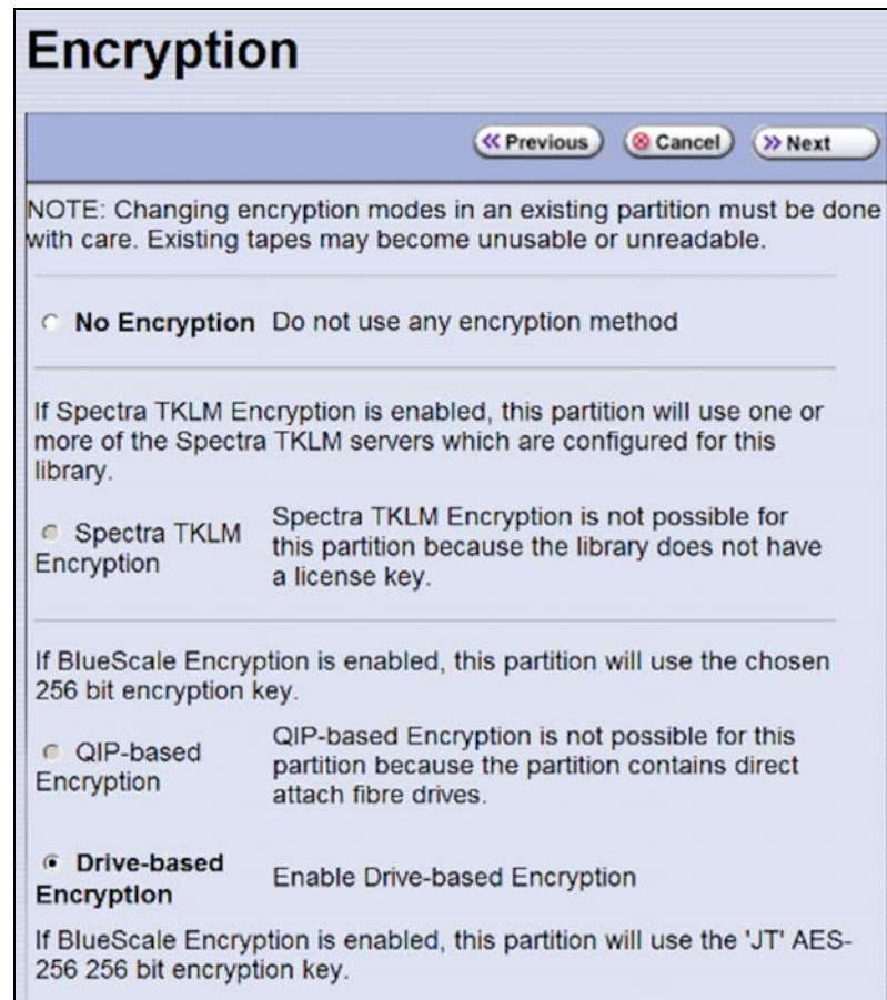
Figure 117 Select whether to use encryption in the partition.
