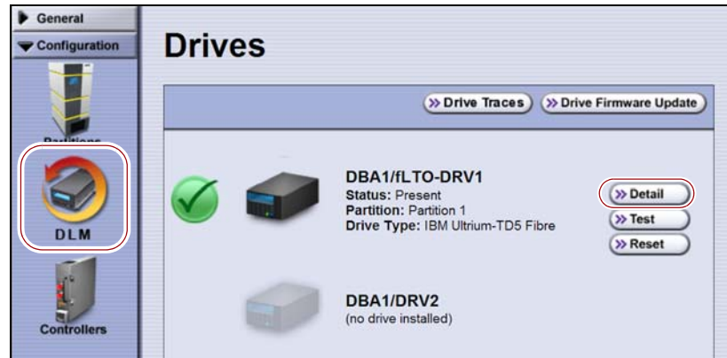
Figure 184 Select Detail to view detailed information about a drive.
