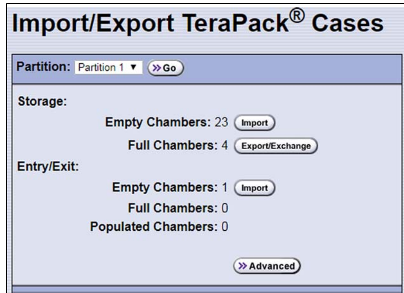
Figure 140 Use the Import/Export TeraPack Cases screen to export or exchange magazines (storage partition shown).
