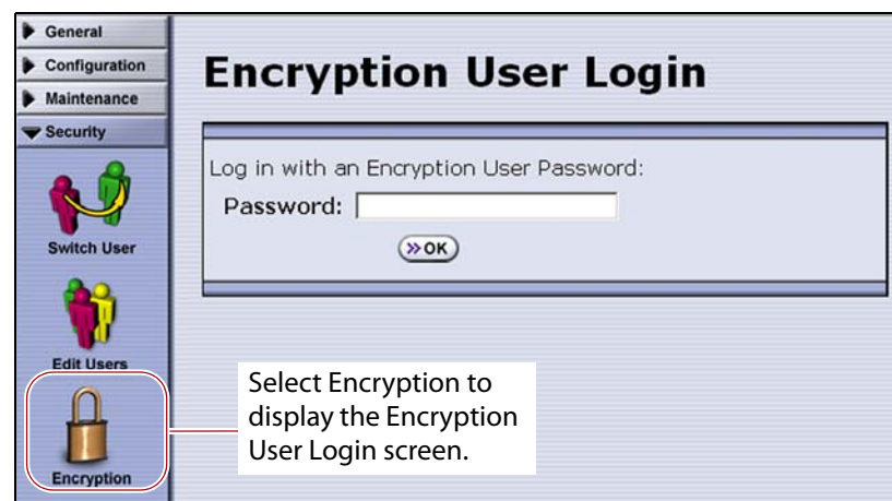
Figure 130 Log into the Encryption feature if you need to change the encryption setting for the partition.
