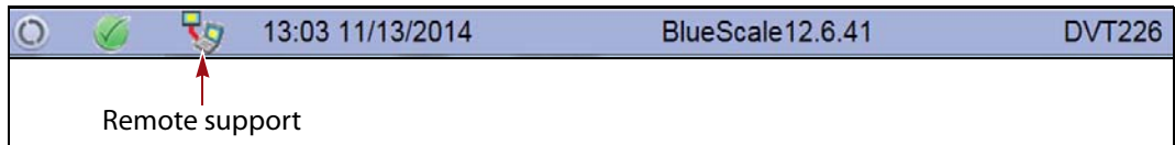
Figure 38 The Remote Support icon in the BlueScale status bar.
