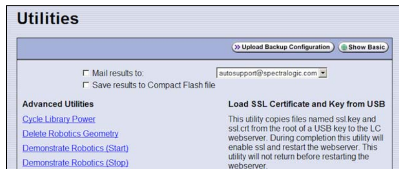
Figure 59 Use the Load SSL Certificate and Key from USB utility to load the security certificate onto the library.
