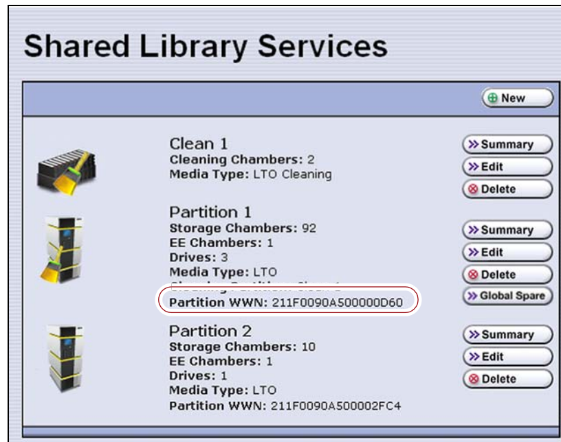
Figure 95 The WWN assigned to the partition.
