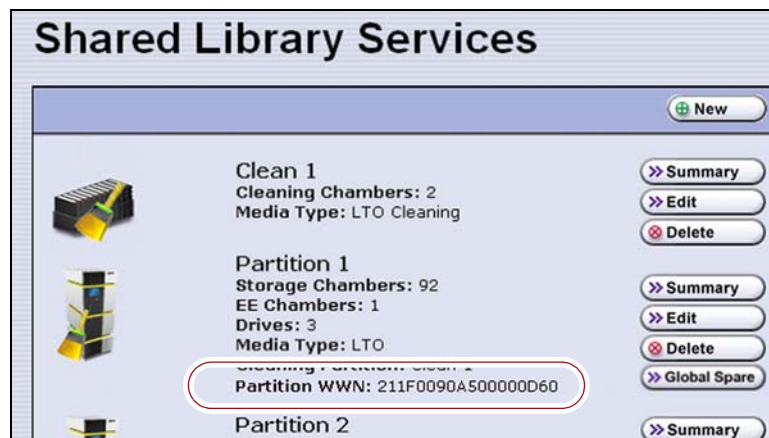
Figure 26 The WWN assigned to the partition.
