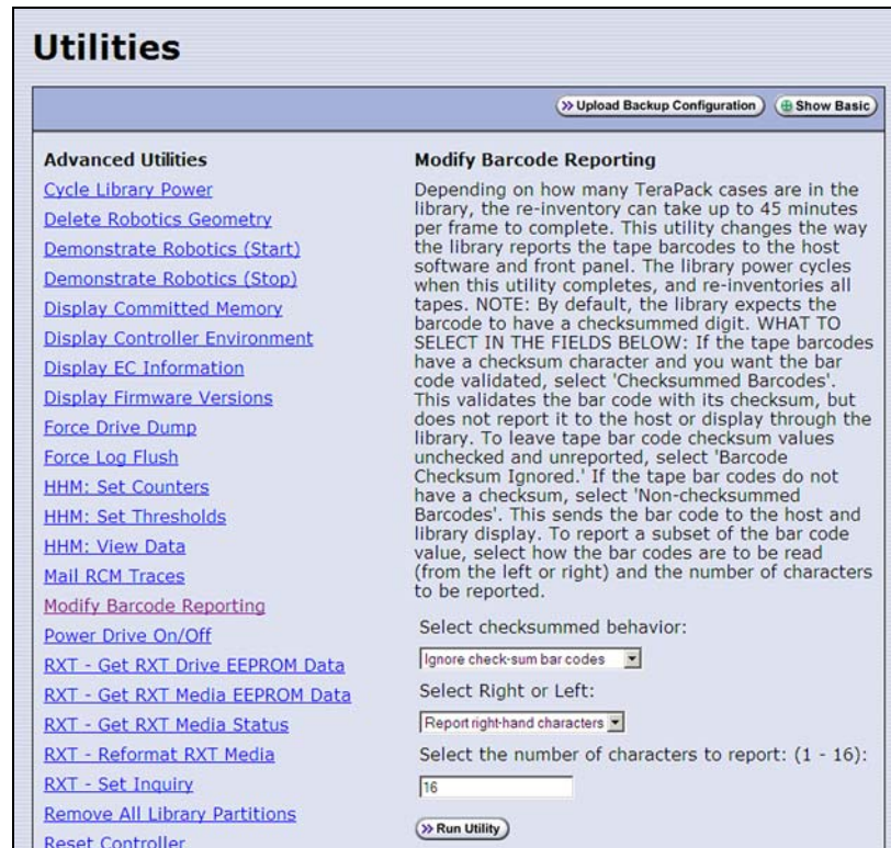
Figure 64 Use the Modify Barcode Reporting utility to change how the library handles barcode labels.
