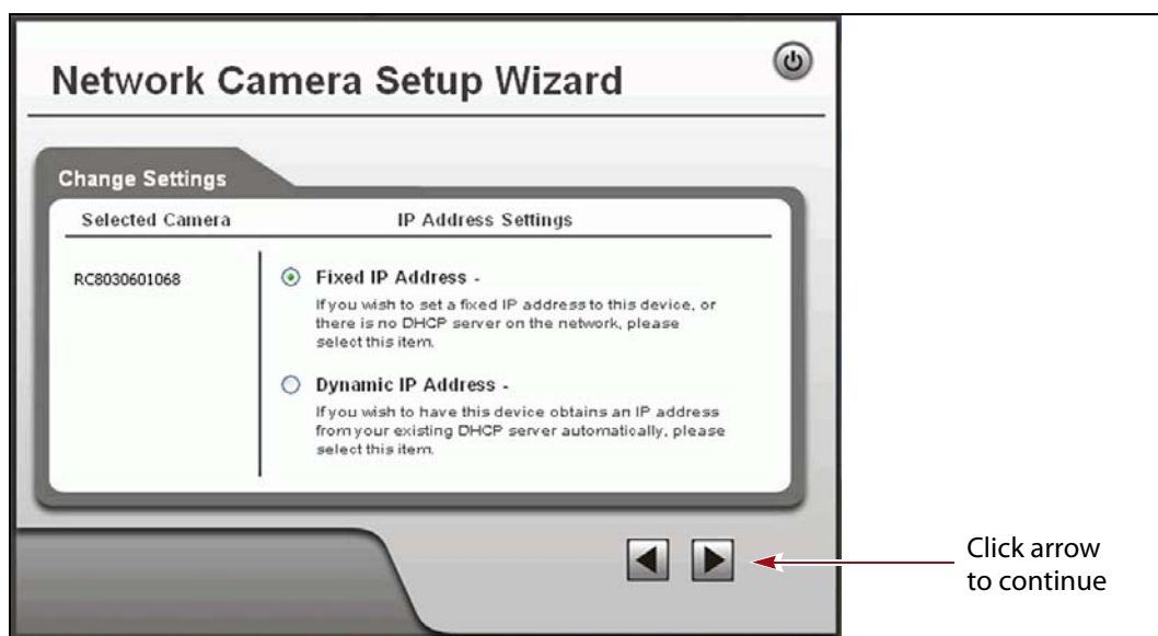
Figure 222 Select Fixed IP Address to configure the IP address for the camera.
