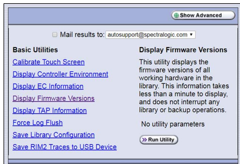
Figure 274 Select the Display Firmware Versions utility.
