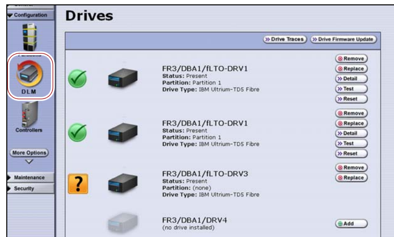
Figure 183 Enabling DLM changes the Drive icon in the Configuration toolbar.
