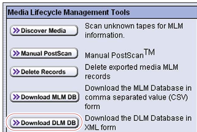
Figure 183 Click Download DLM DB to export the DLM database as an XML file.
