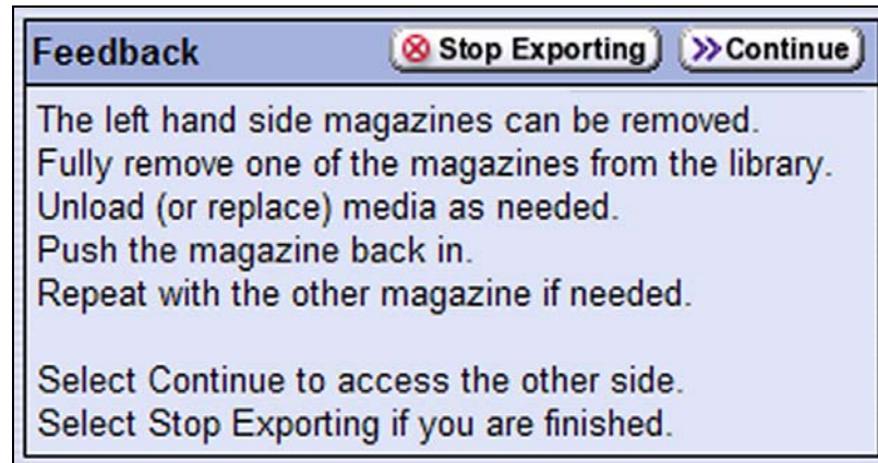
Figure 140 Do not click Continue until after you unload the magazines on the left side of the library.
