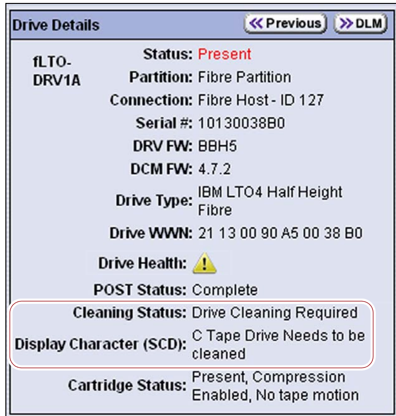
Figure 304 The Drive Details screen shows that cleaning is required.
