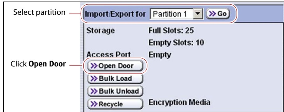
Figure 308 Select the partition and then click Open Door to open the access port.
