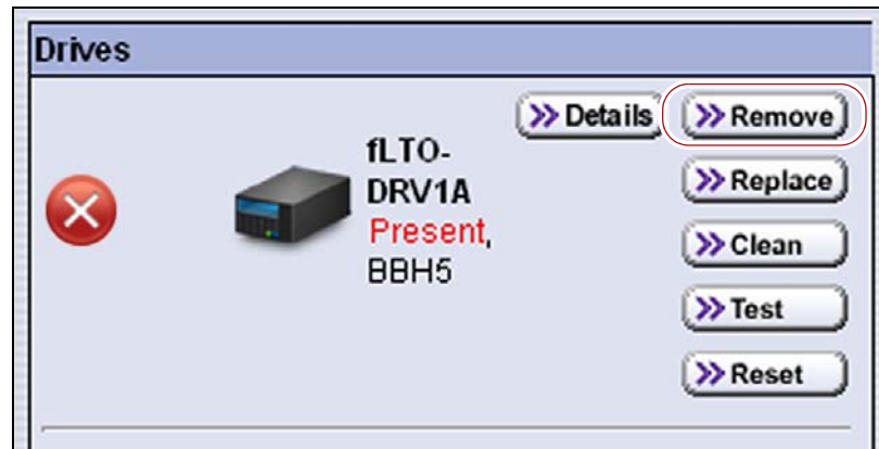
Figure 318 Click Remove next to the drive you want to permanently remove from the library.
