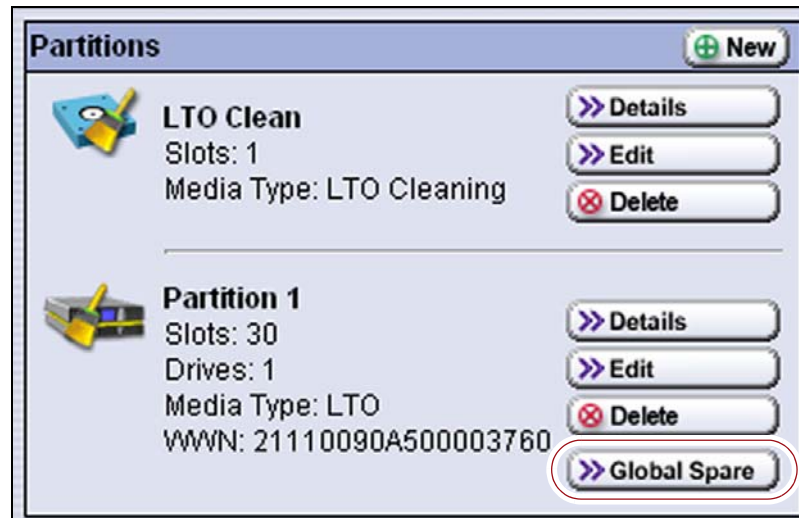
Figure 273 Click Global Spare to begin the process of replacing a partition drive with a Global Spare drive.
