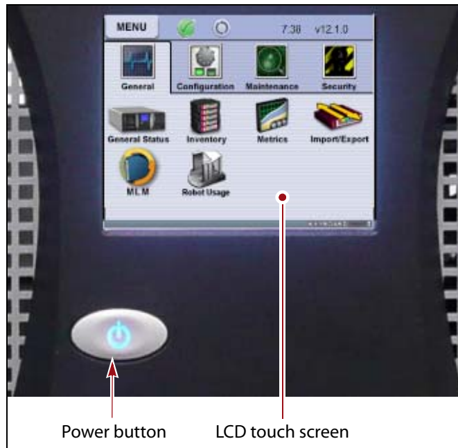
Figure 6 The library operator panel displaying the BlueScale user interface.
