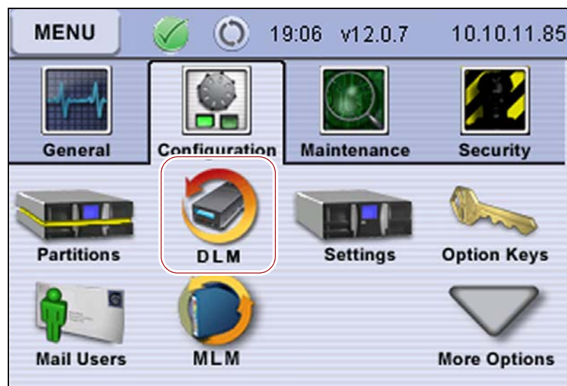
Figure 176 Enabling DLM changes the Drive icon to a DLM icon in the Configuration menu.
