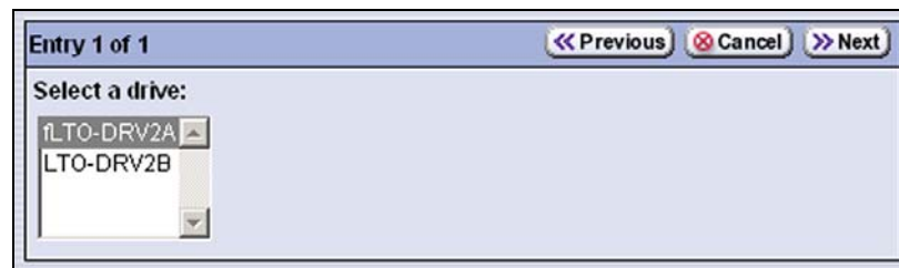
Figure 270 Select the drive from which you want to retrieve the dump file.
