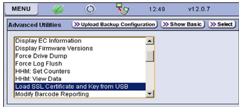
Figure 70 Use the Load SSL Certificate and Key from USB utility to load the security certificate onto the library.
