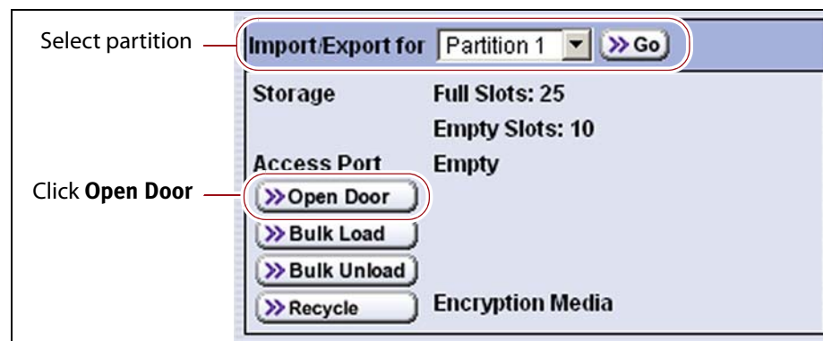
Figure 131 Select the partition and then click Open Door to open the access port.
