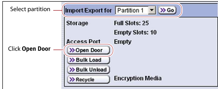
Figure 136 Select the partition and then click Open Door to open the access port.
