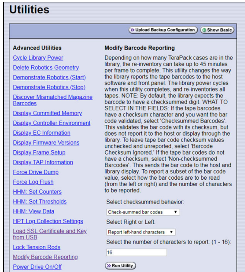
Figure 74 Use the Modify Barcode Reporting utility to change how the library handles barcode labels.
