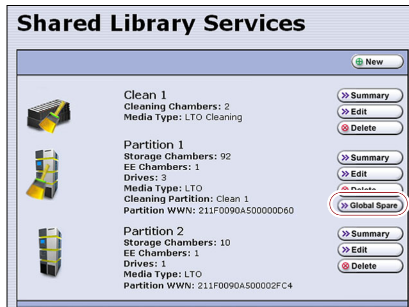
Figure 259 Click Global Spare to begin the process of replacing a partition drive with a Global Spare drive.
