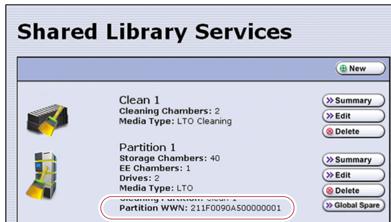
Figure 34 The WWN assigned to the partition.
