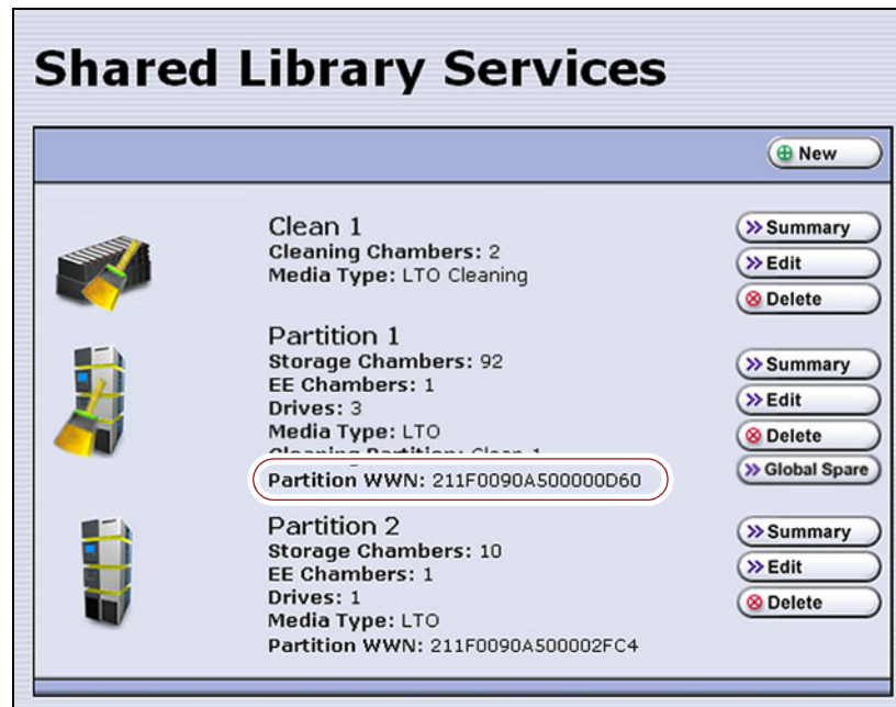
Figure 105 The WWN assigned to the partition.
