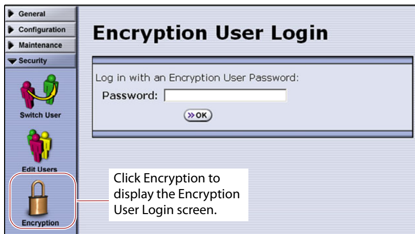
Figure 140 Log into the Encryption feature if you need to change the encryption setting for the partition.
