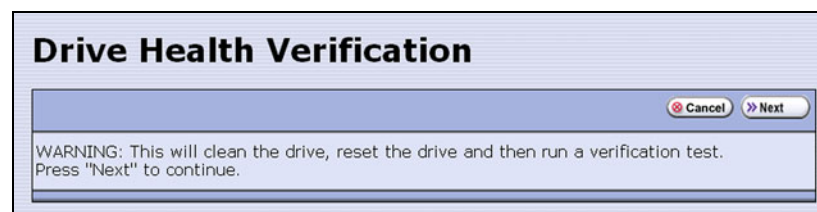
Figure 269 Click Next on the Drive Health Verification screen to begin the verification process.
