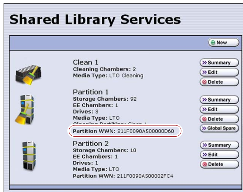
Figure 78 The WWN assigned to the partition.
