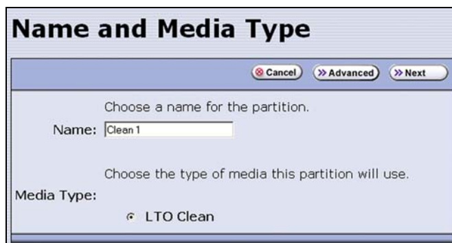
Figure 104 The Name and Media Type screen for a cleaning partition.
