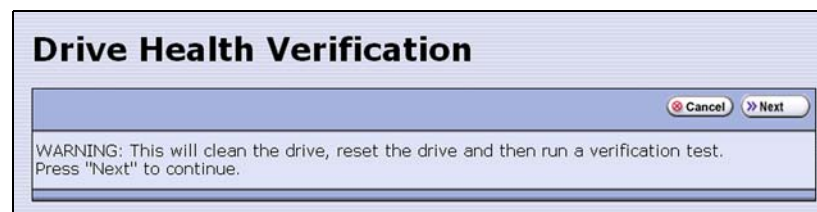
Figure 208 Click Next on the Drive Health Verification screen to begin the verification process.
