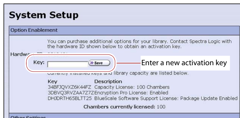
Figure 42 Enter the keys in the Option Enablement pane of the System Setup screen.
