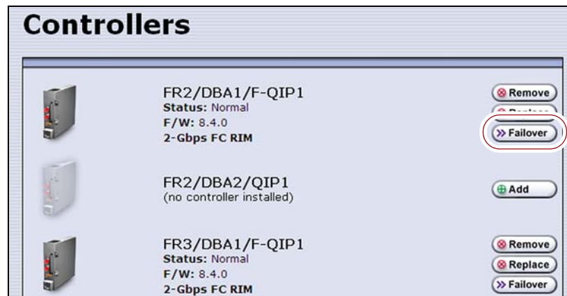
Figure 53 The Controllers screen before the failover controller is selected.
