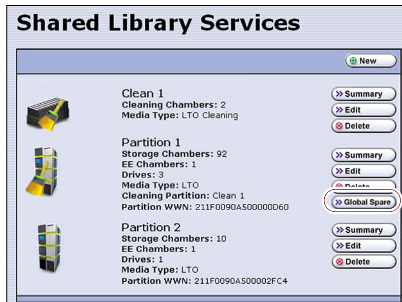
Figure 198 Click Global Spare to begin the process of replacing a partition drive with a Global Spare drive.
