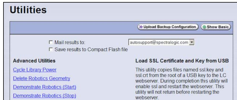
Figure 50 Use the Load SSL Certificate and Key from USB utility to load the security certificate onto the library.
