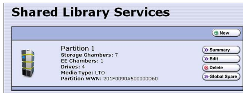
Figure 80 Click New on the Shared Library Services screen to begin creating the cleaning partition.
