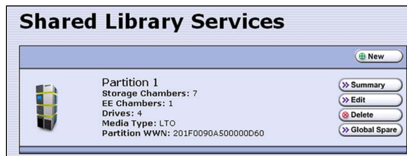
Figure 84 Click New on the Shared Library Services screen to begin creating the storage partition.
