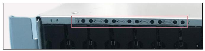
Figure 208 The top left section of the front of the Gen2 X chassis showing system status LEDs.
