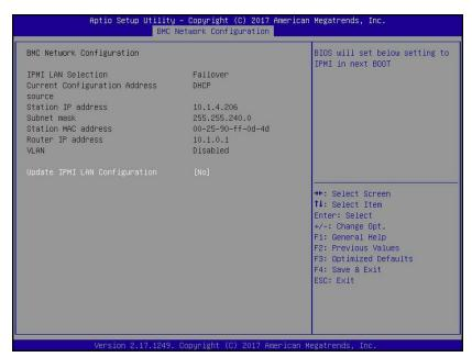
**Figure 267** The BMC Configuration screen.
