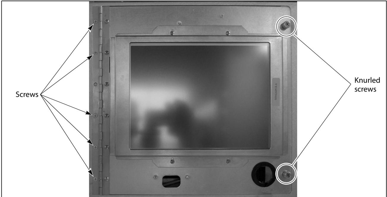
**Figure 24** Attach the LCD panel to the chassis.
