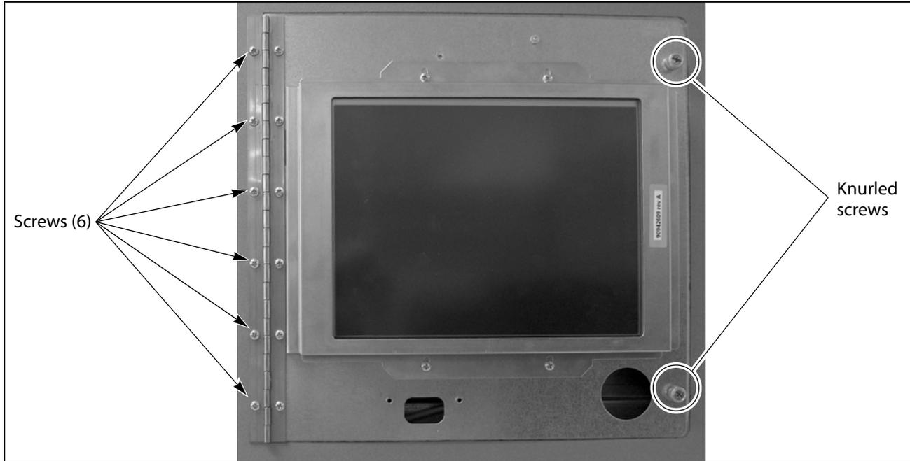
**Figure 44** Attach the LCD panel to the chassis.
