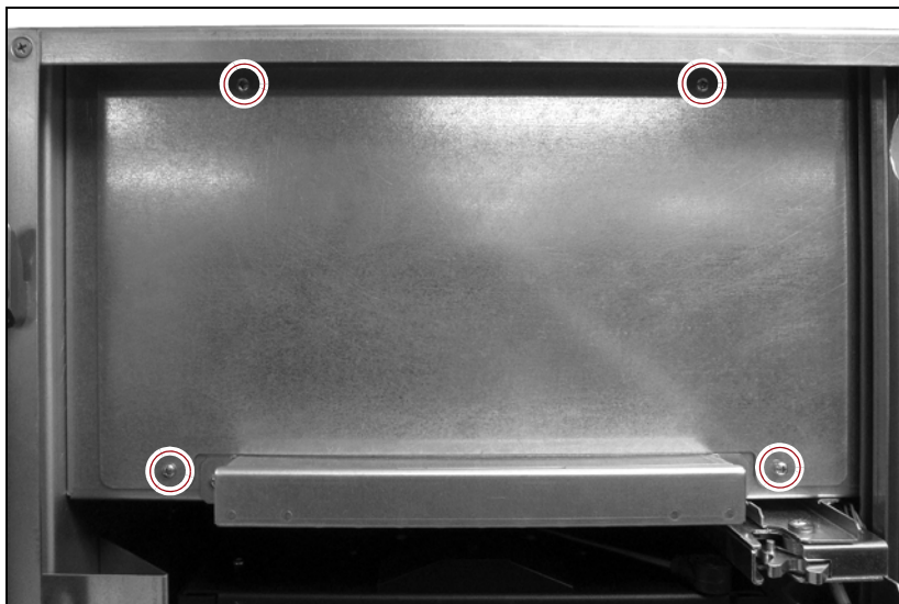
Figure 20 Remove the carousel motor compartment cover.
