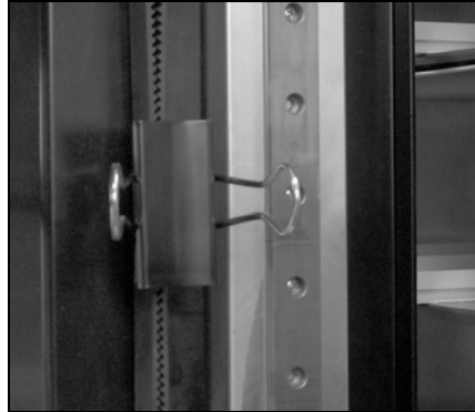
Figure 20 Clamp the VAX belt to hold the transporter.
