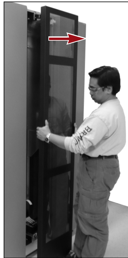
Figure 10 Lift the panel out and away from the frame
