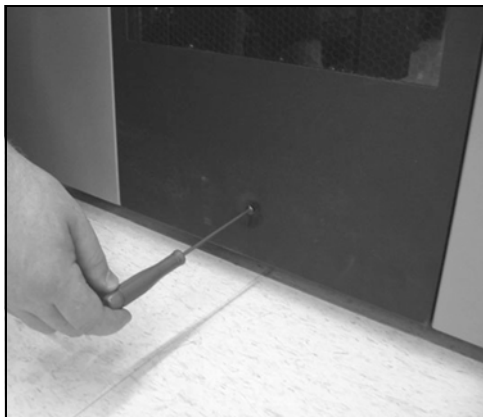
Figure 3 Remove the screw at the bottom of the window panel.
