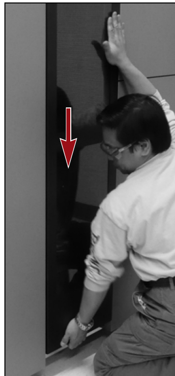
Figure 17 Slide the panel down into place.
