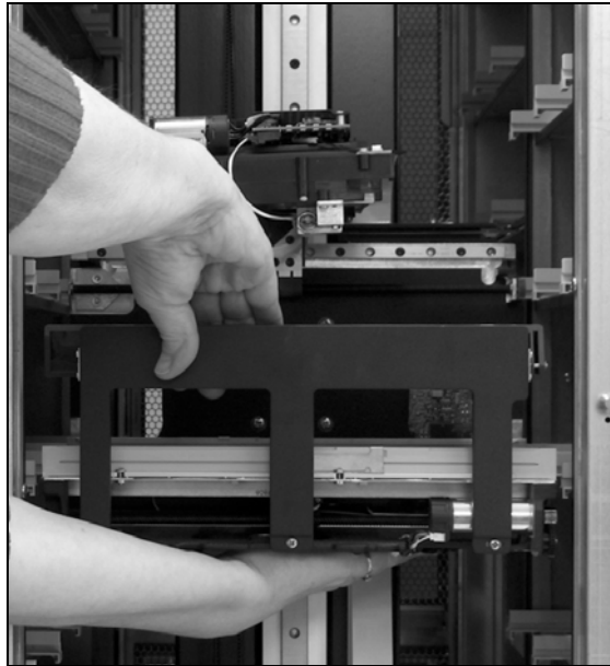
Figure 13 Lift the transporter into the library and onto the mounting bracket.
