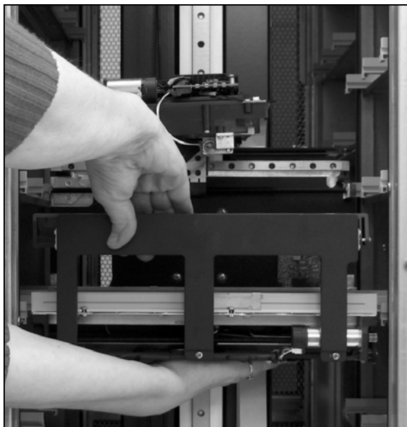
Figure 10 Lift the transporter off its mounting bracket.
