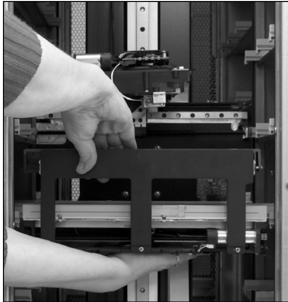
Figure 14 Lift the transporter off of its mounting bracket.
