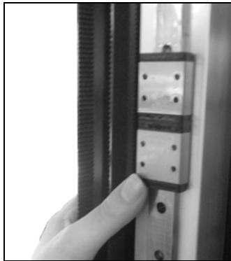
Figure 34 Position bearing mounts above rail joint and let them slide down the rail.
