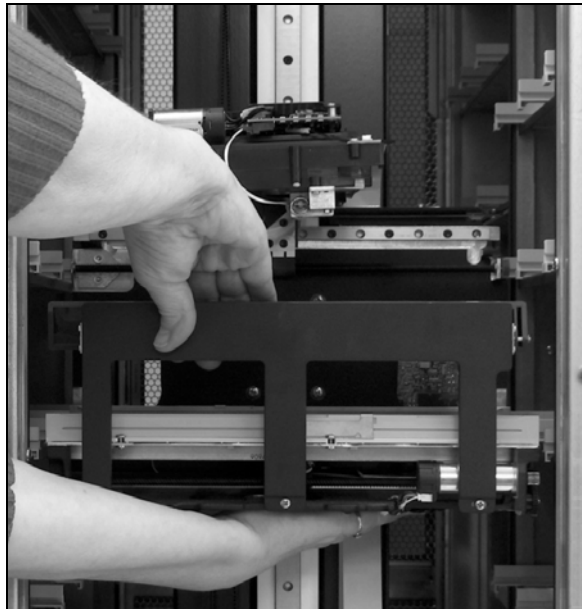
Figure 40 Lift the transporter into the library and onto the mounting bracket.
