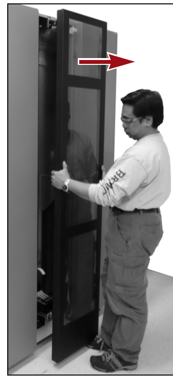
Figure 9 Lift the panel out and away from the frame.
