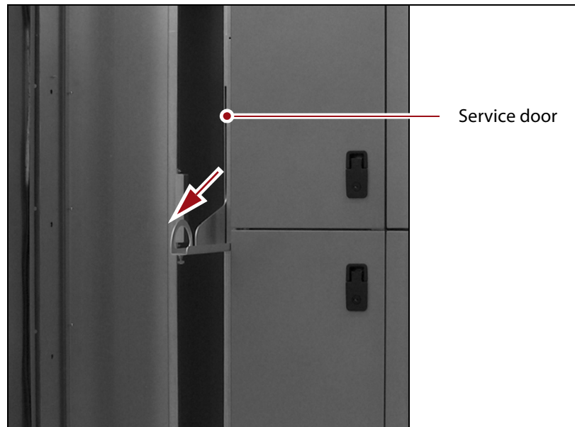
Figure 40 Slide the service bay safety door toward you to its open position.
