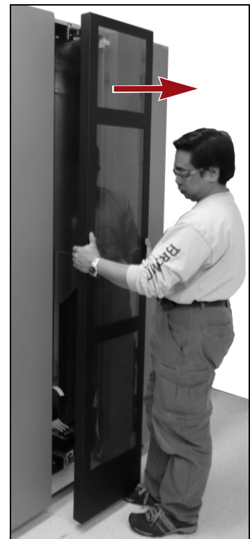
Figure 8 Lift the panel out and away from the frame.
