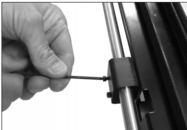
Figure 22 Remove the center rod support.
