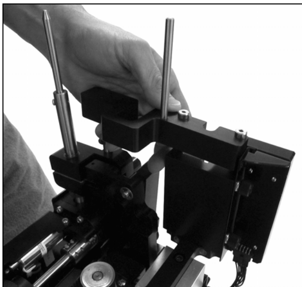
Figure 43 Install the retaining bracket.
