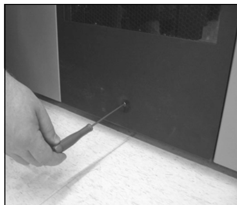
Figure 74 Use #2 Phillips screwdriver to install the screw at the bottom of the side panel.
