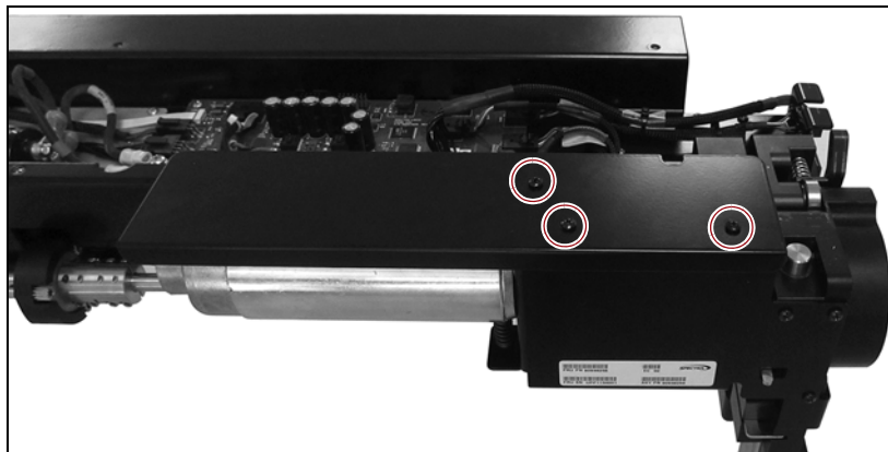
Figure 21 Optionally, remove the HAX motor cover on the rear of the VAX column.
