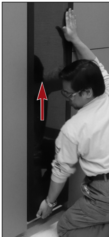
Figure 7 Slide the panel up to disengage the hangers.
