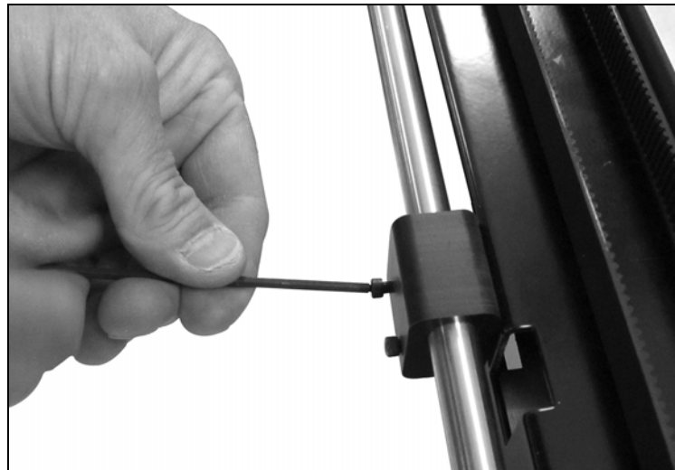
Figure 48 Install the center rod support.
