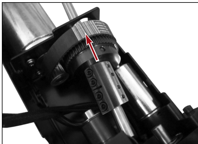
Figure 34 Push the bearing through the bracket.
