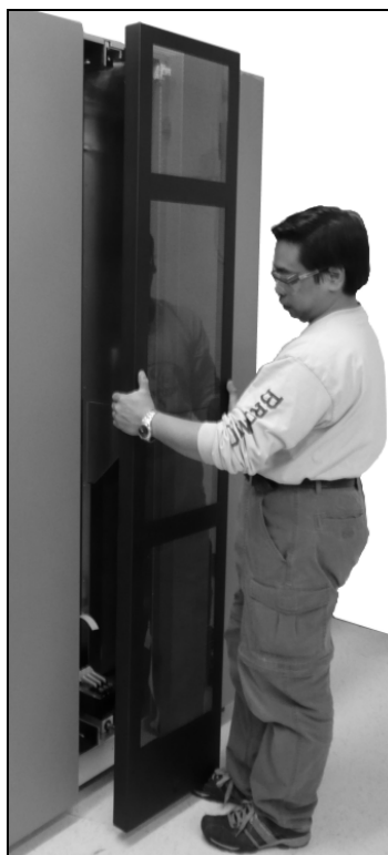
Figure 72 Lift the panel onto the hooks at the top of the opening.
