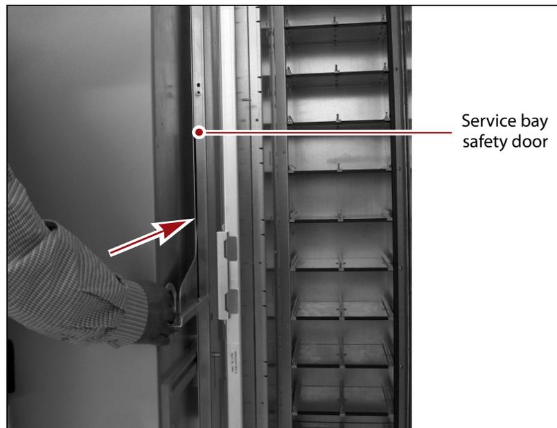
**Figure 8** Slide the service bay safety door inward to its closed position.
