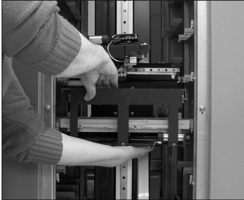
**Figure 22** Lift the transporter off its mounting bracket and remove it from the library.
