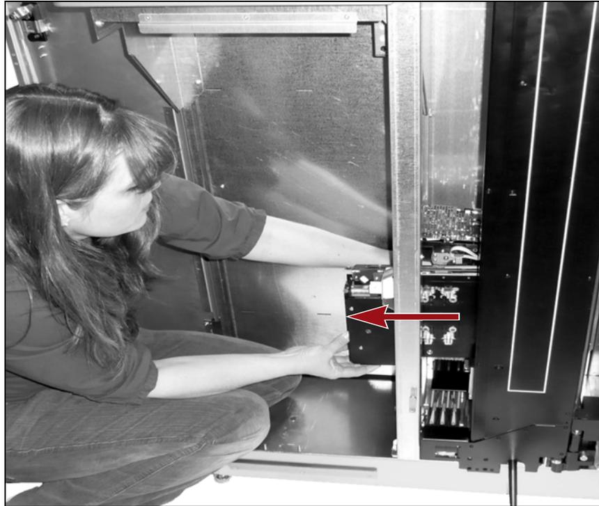
**Figure 17** Lift the transporter off its mounting bracket and remove it from the library.
