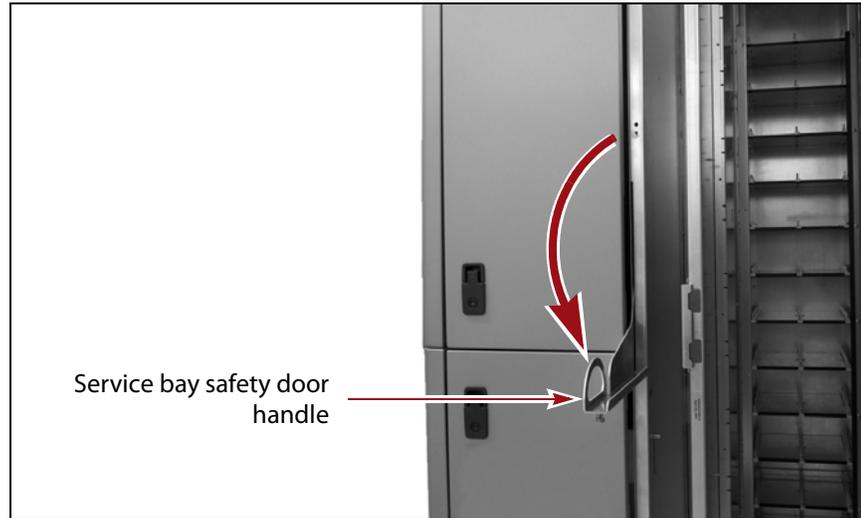
**Figure 7** Rotate the handle on the service bay safety door down to horizontal (service bay safety door for Robot 2 shown).
