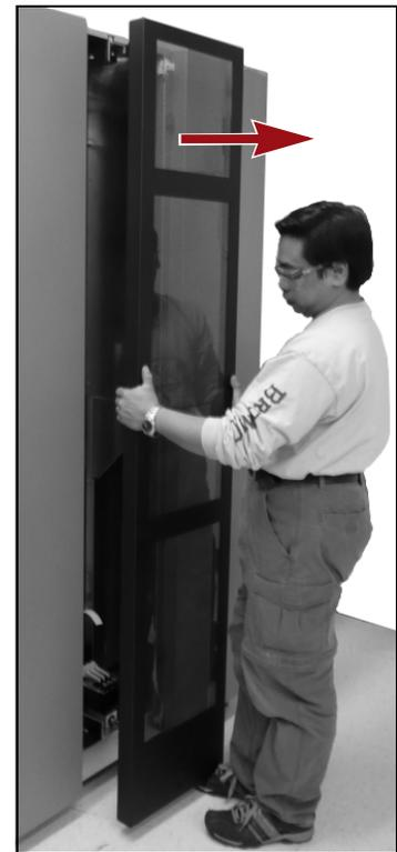
**Figure 11** Lift the panel out and away from the frame.
