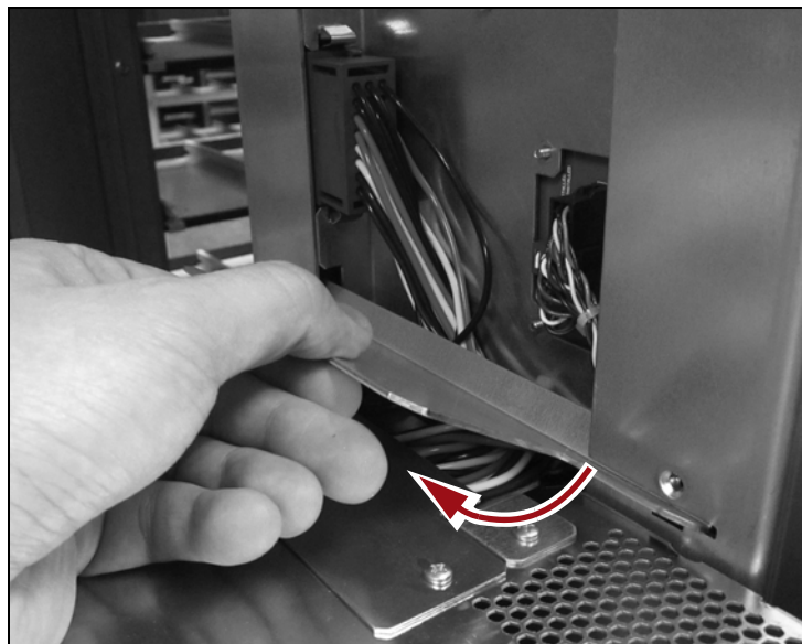
Figure 38 Pull the bay support shelf out of the library.
