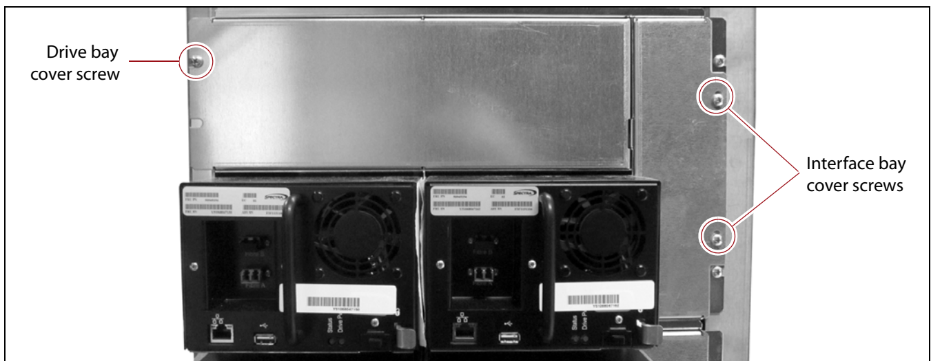
Figure 8 Remove drive bay or interface bay cover screws
