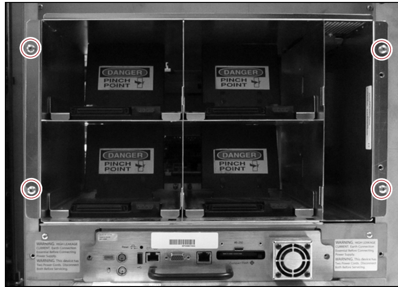
Figure 16 Remove the DBA screws.
