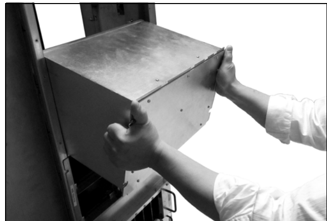
Figure 47 Angle the interior side of the TBA upwards during removal.
