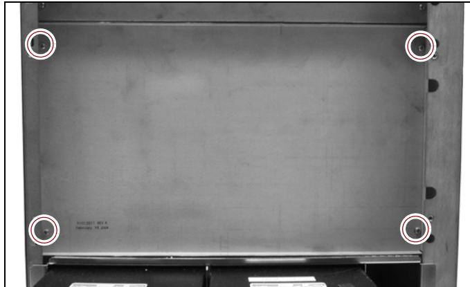
Figure 9 Remove the shelf cover screws.
