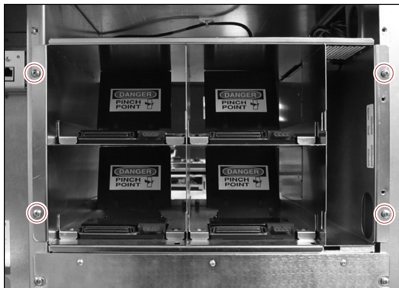
Figure 42 Remove the DBA screws.
