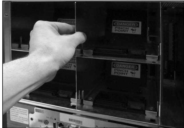
Figure 19 Remove the DBA from the library.
