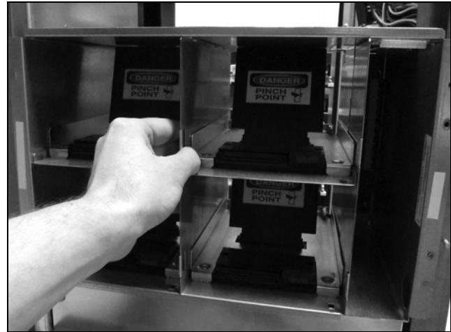
Figure 44 Remove the DBA from the library.
