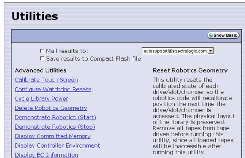
Figure 62 Select the Reset Robotics Geometry utility.
