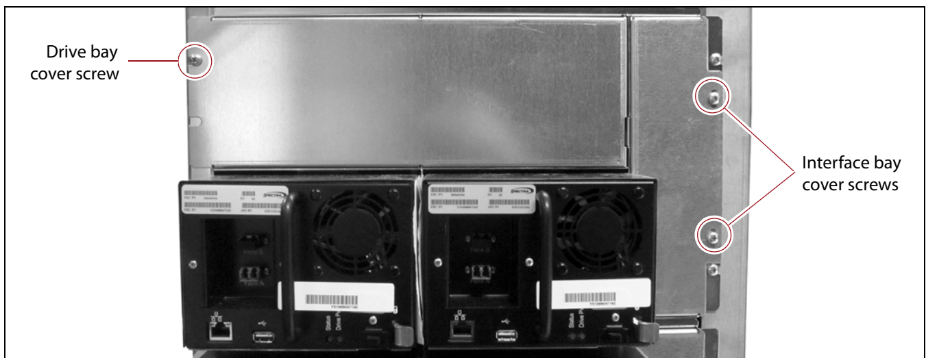
Figure 36 Remove drive bay or interface bay cover screws
