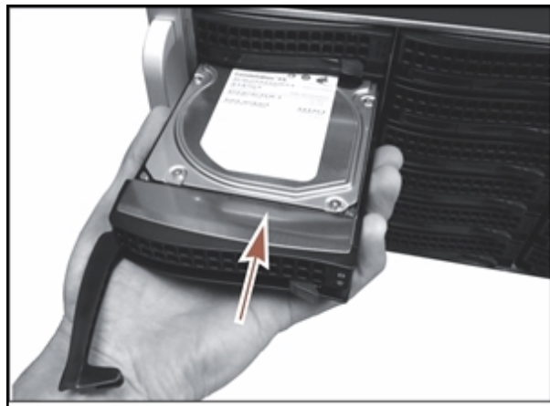
Figure 42 Install the drive into the chassis.
