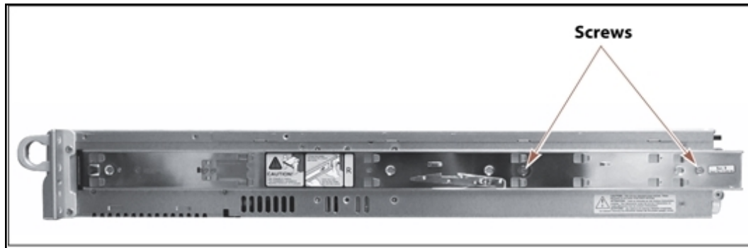
Figure 36 Install the inner rail screws on the BlackPearl NAS 2U chassis.
