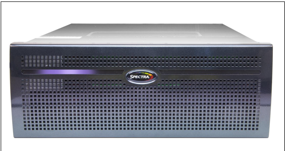
Figure 1 A 4U BlackPearl chassis with front bezel and visual status beacon.
