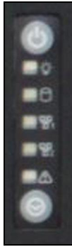
Figure 143 The top right section of the front of the Gen2 S Series chassis, with the front bezel removed, showing system status LEDs.
