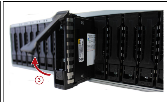
Figure 201 Remove the drive sled with drive blank and insert the drive sled with drive.
