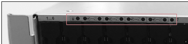
Figure 142 The top left section of the front of the Gen2 X chassis (front bezel removed) showing system status LEDs.
