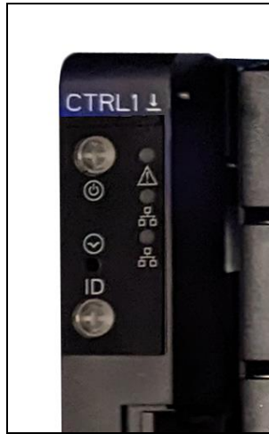
Figure 141 The Gen3 H Series chassis system status LEDs.
