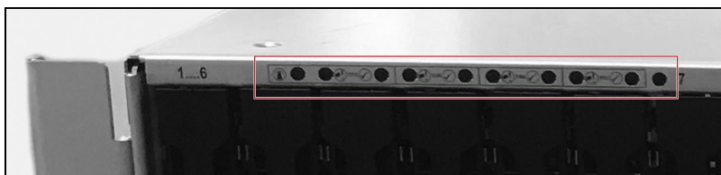
Figure 94 The top left section of the front of the Gen2 X chassis (front bezel removed) showing system status LEDs.
