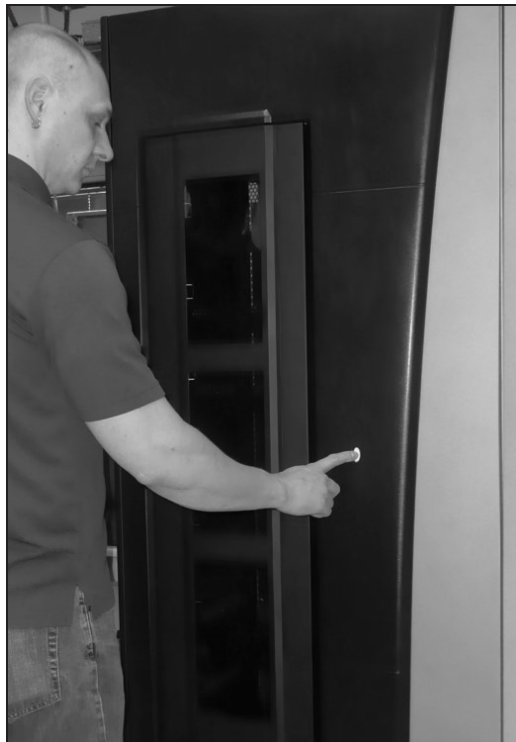
Figure 266 Press the door release button to open the door.
