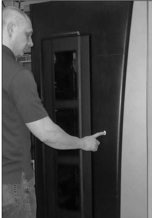
Figure 247 Press the door release button to open the door.
