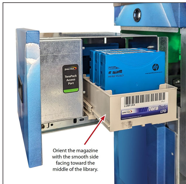
Figure 233 Insert a magazine into the TAP, making sure that it is correctly oriented.
