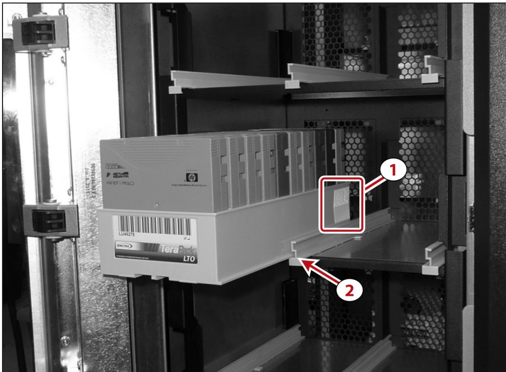
Figure 248 Insert the magazine into the bulk TAP carousel, making sure that it is correctly positioned.
