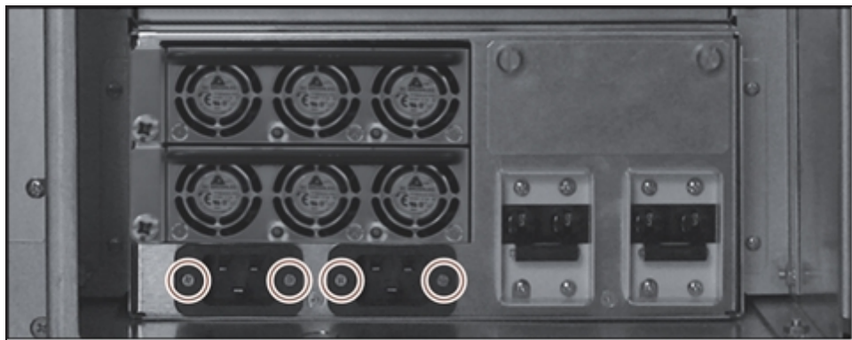
Figure 70 Remove the screws on the service frame expansion power module.
