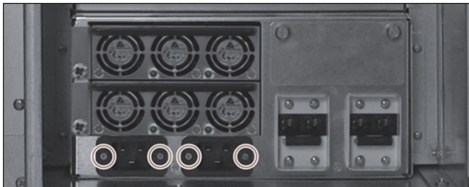
Figure 91 Remove the screws on the service frame expansion power module.
