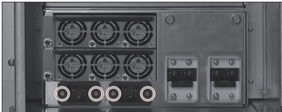
Figure 92 Remove the screws on the service frame expansion power module.
