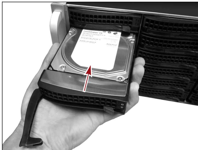
Figure 6 Install the drive into the BlackPearl gateway.
