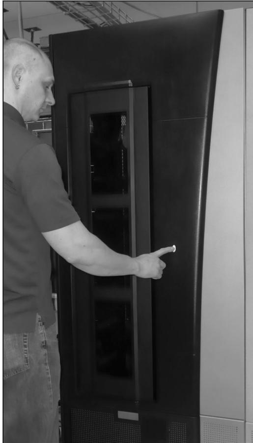
**Figure 266** Press the door release button to open the door.
