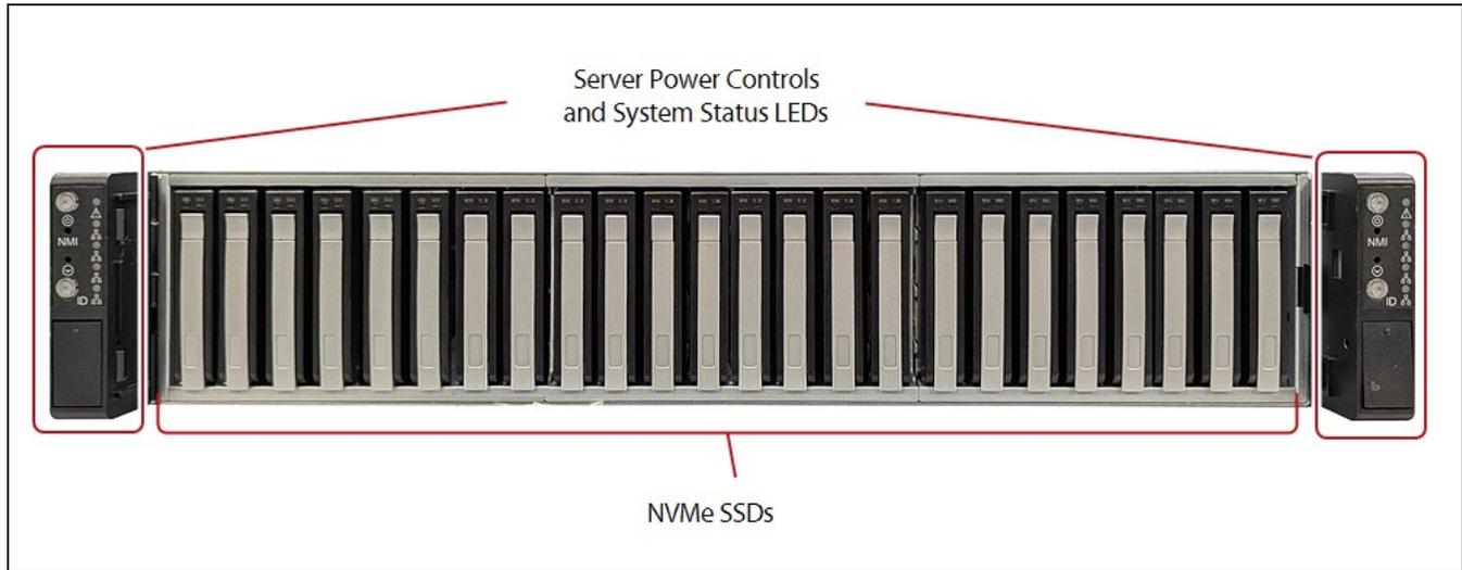
**Figure 2** The front view of the Gen3 F Series BlackPearl gateway (front bezel removed).
