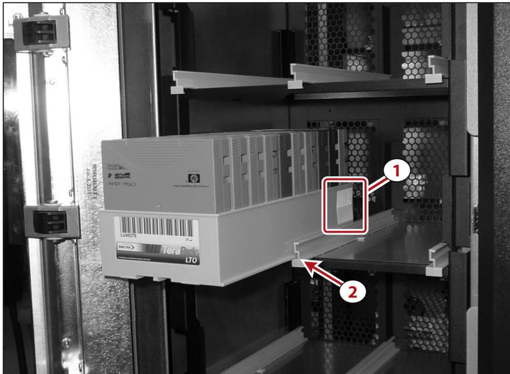
**Figure 267** Insert the magazine into the bulk TAP carousel, making sure that it is correctly positioned.
