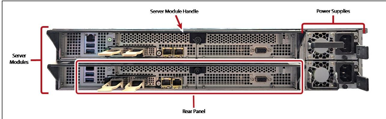
**Figure 3** The rear view of the Gen3 F Series BlackPearl gateway.
