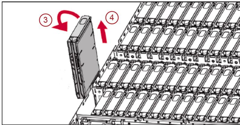
**Figure 314** Remove the drive from the BlackPearl chassis.
