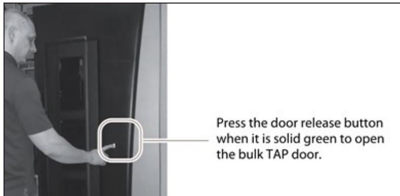
**Figure 276** Press the door release button to open the door.
