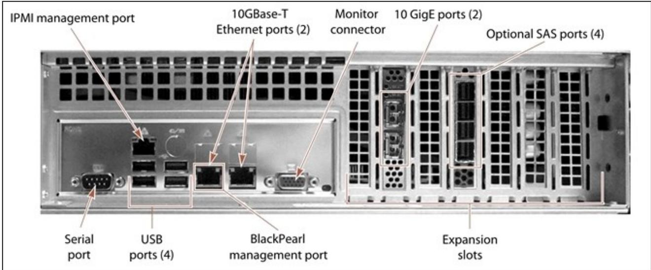
**Figure 21** The Gen1 S Series BlackPearl rear panel components.
