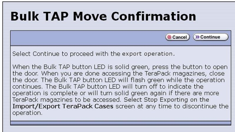
**Figure 282** Read the instructions on the Bulk TAP Move Confirmation screen, then click **Continue**.
