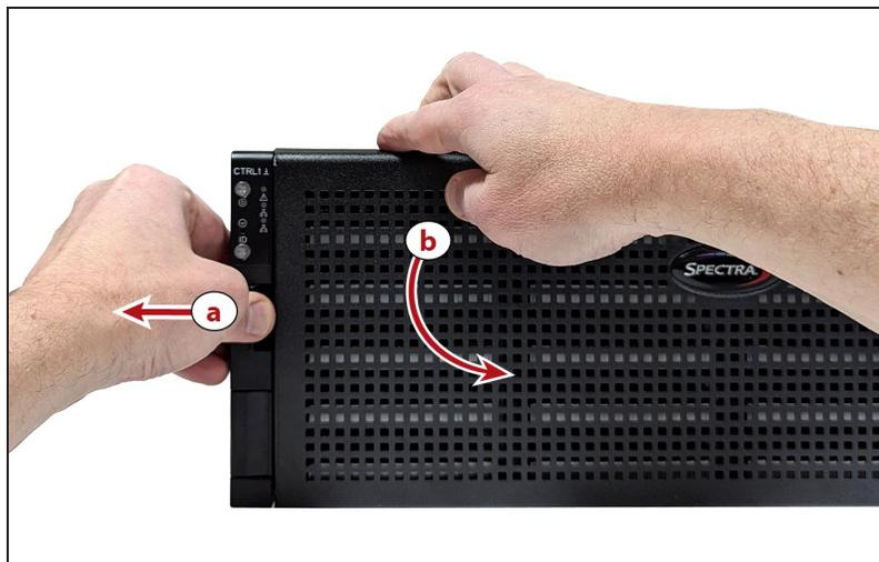
**Figure 296** Remove the front bezel.
