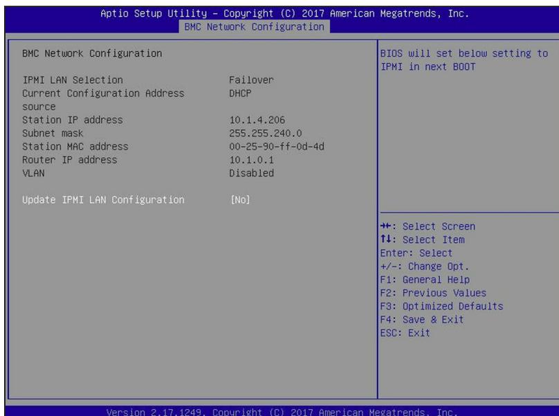
**Figure 352** The BMC Configuration screen.
