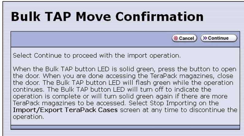
**Figure 265** Read the instructions on the Bulk TAP Move Confirmation screen, then click **Continue**.
