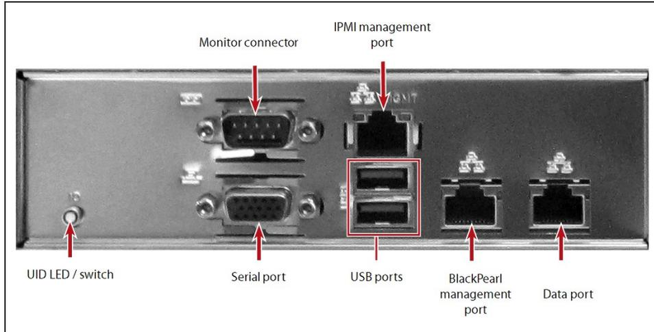
**Figure 14** The Gen2 S Series and Gen 2 V Series BlackPearl rear panel components.
