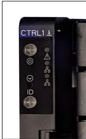
**Figure 171** The Gen3 H Series chassis system status LEDs.
