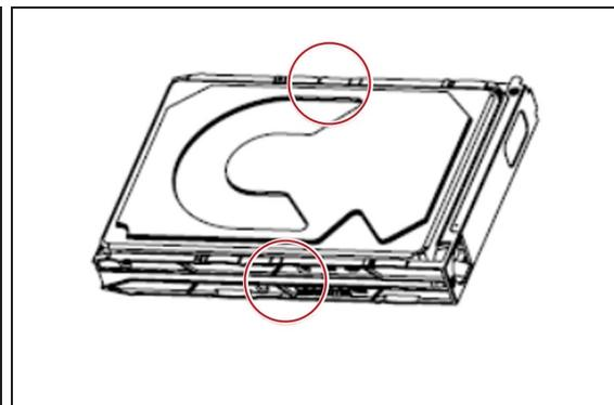
**Figure 316** The drive installed in the drive sled.
