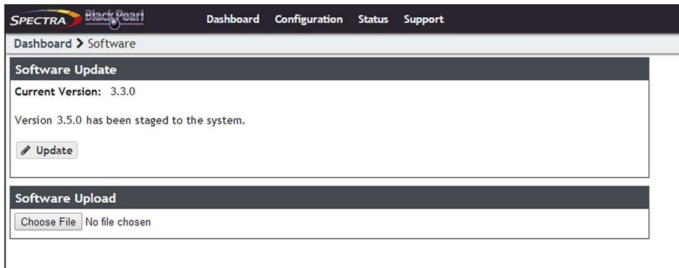
**Figure 293** The Software Update screen with an available software package listed.
