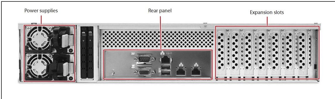
**Figure 13** The rear view of the Gen2 V Series BlackPearl 2U gateway.
