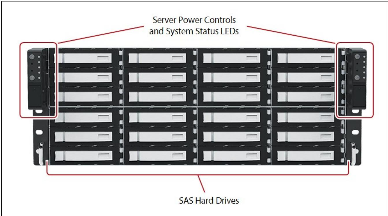
**Figure 5** The front view of the Gen3 H Series BlackPearl gateway (front bezel removed).
