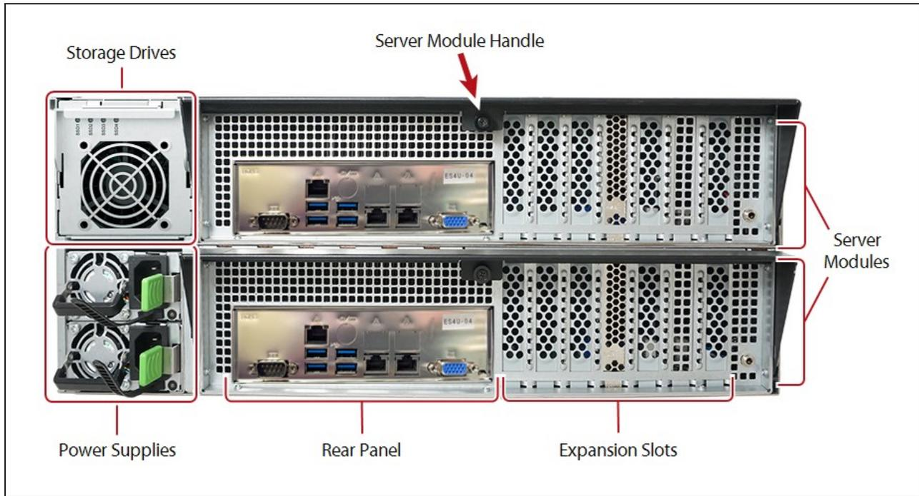
**Figure 6** The rear view of the Gen3 H Series BlackPearl gateway.
