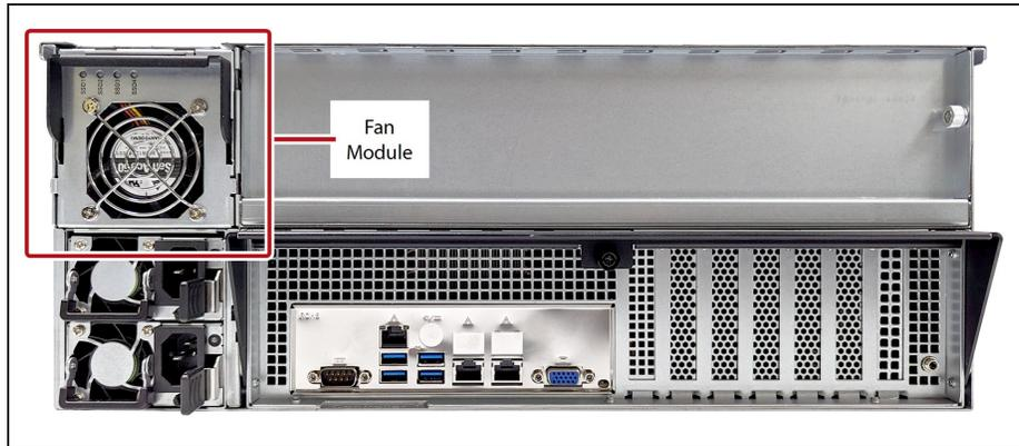
**Figure 305** The NVMe drive fan module.
