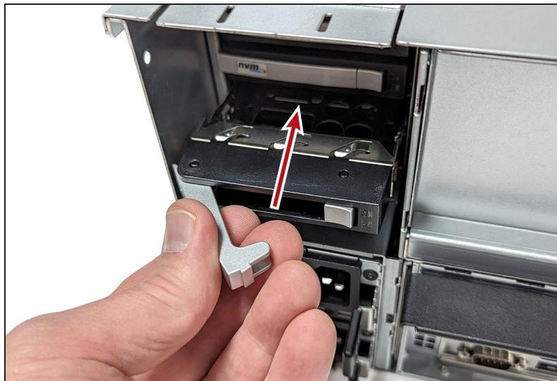
**Figure 311** Insert drive into chassis.
