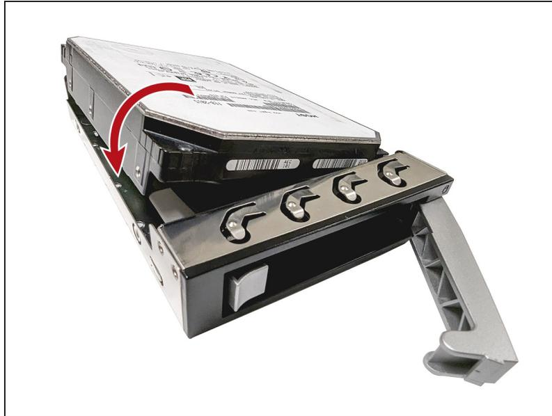
**Figure 300** Unlock the drive sled.
