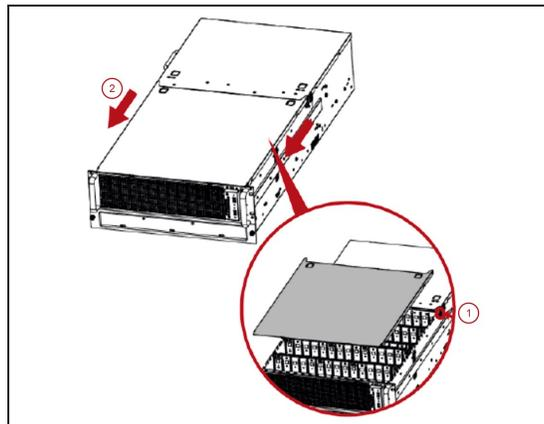
**Figure 313** Remove the front top cover.
