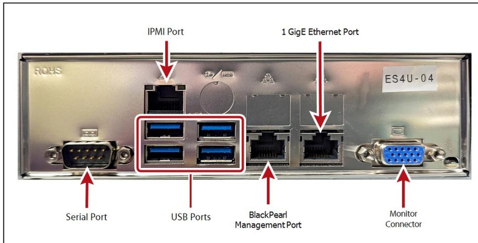
**Figure 7** The Gen3 H Series BlackPearl rear panel components.
