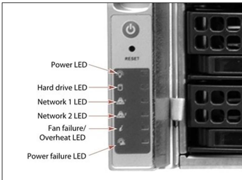
**Figure 175** The left side of the front of the Gen1 S Series chassis showing system status LEDs.
