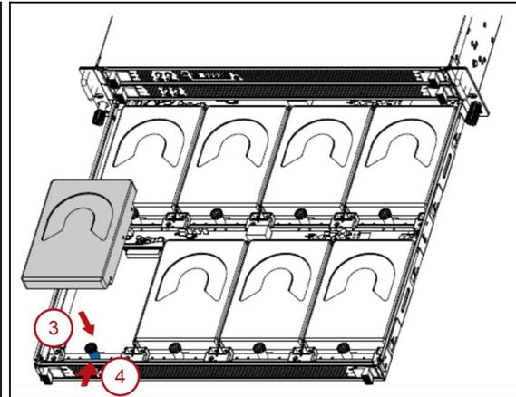
**Figure 318** Install the drive.
