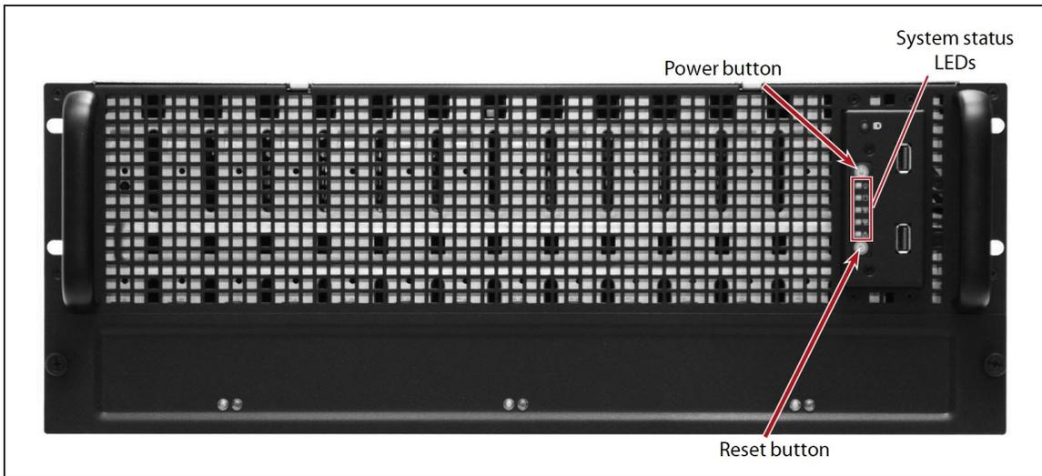
**Figure 10** The front view of the Gen2 S Series BlackPearl 4U gateway (front bezel removed).
