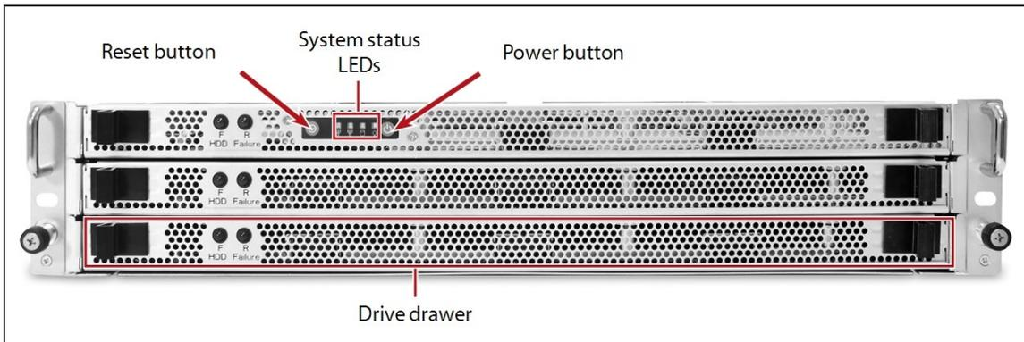
**Figure 11** The front view of the Gen2 V Series BlackPearl 2U gateway (front bezel removed).
