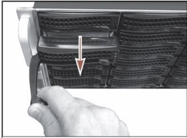
**Figure 322** Pull the sled out of the gateway.
