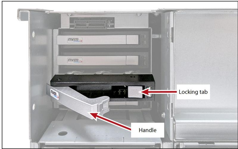
**Figure 307** Unlock the drive sled.
