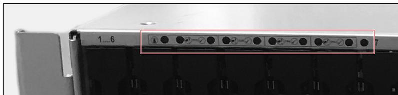
**Figure 172** The top left section of the front of the Gen2 X chassis (front bezel removed) showing system status LEDs.
