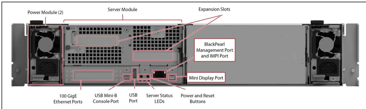
**Figure 9** The rear view of the Gen2 X Series BlackPearl gateway.
