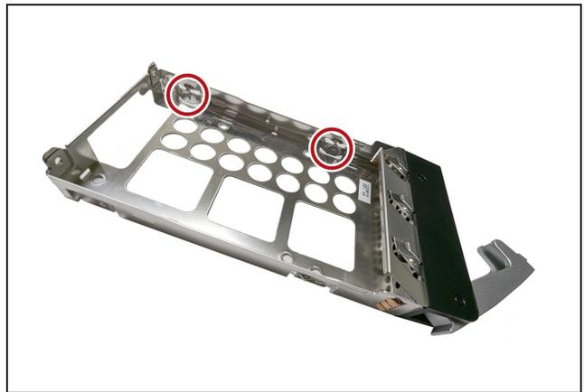
**Figure 309** PEMs on right side of sled.
