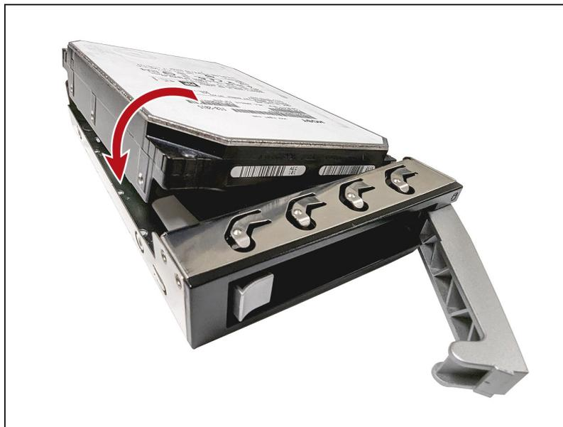
**Figure 301** Insert drive into chassis.
