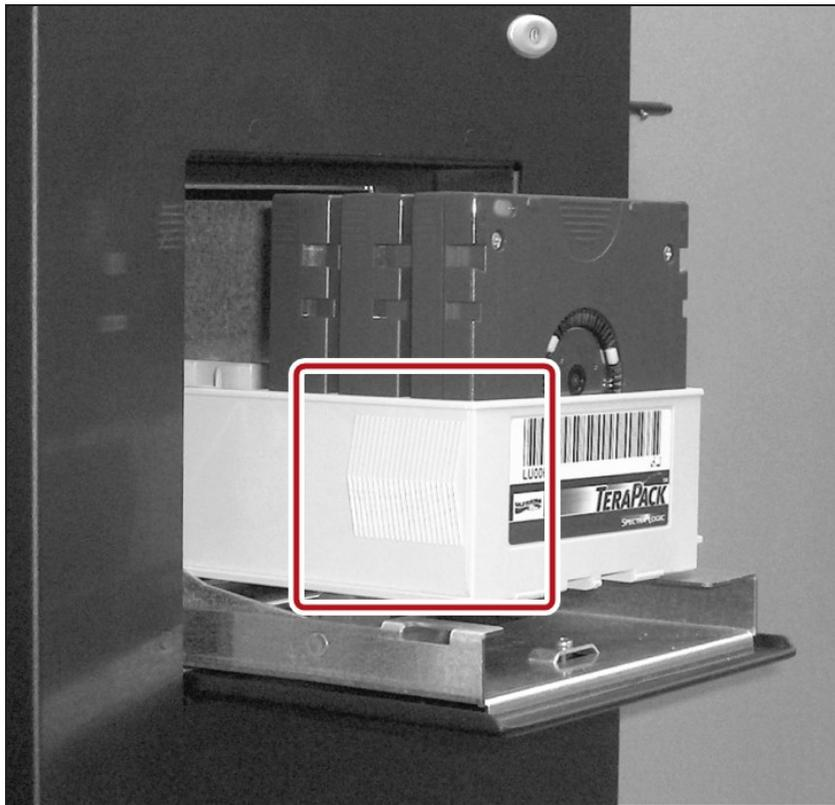
**Figure 264** Insert a magazine into the TAP, making sure that it is correctly oriented.
