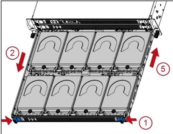
**Figure 317** Remove the drive tray.
