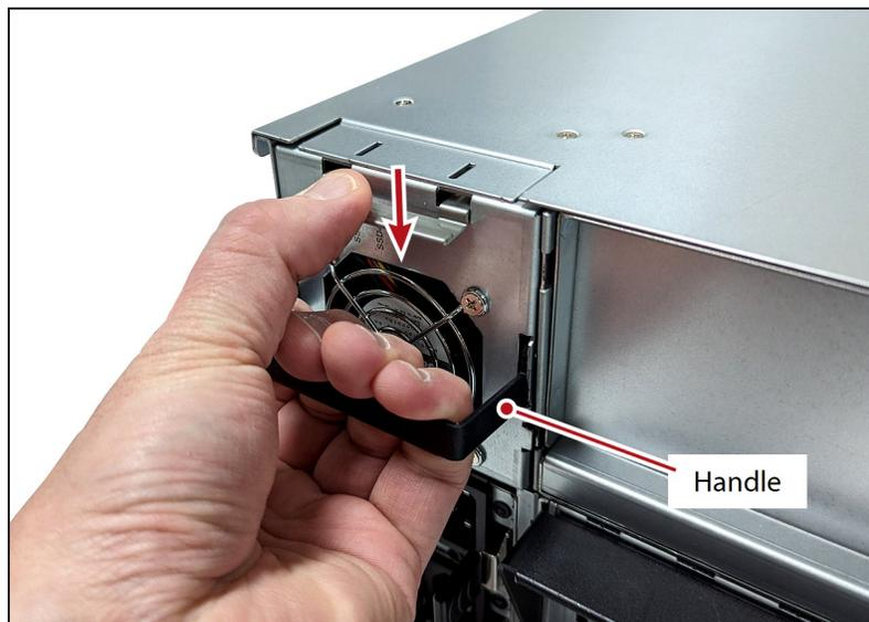
**Figure 306** Remove the NVMe drive fan module.
