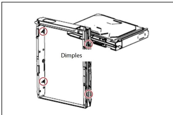
**Figure 315** Match the dimples on the drive sled to the dimples on the drive.
