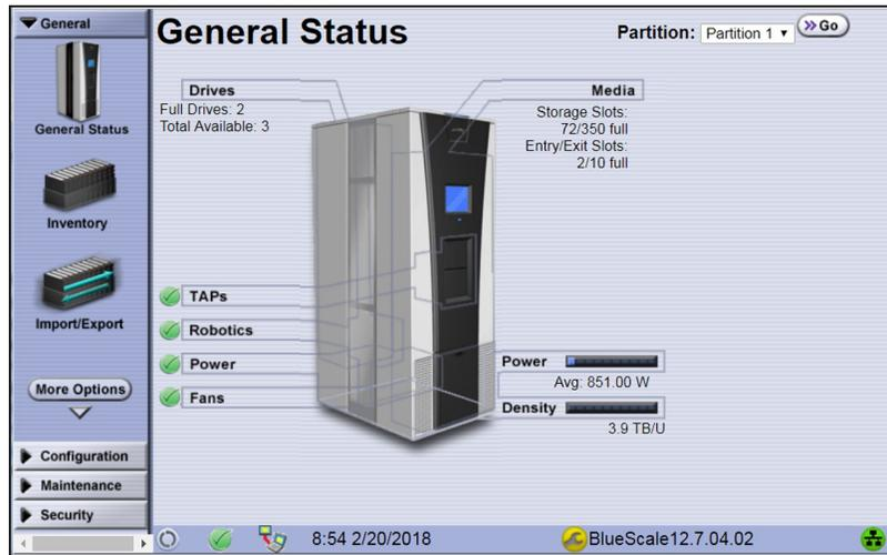
**Figure 279** The BlueScale user interface General Status screen for a Spectra TeraPack-based tape library.
