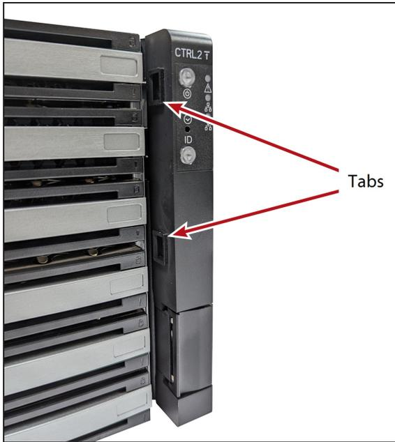
**Figure 302** Tabs on the side of power control.
