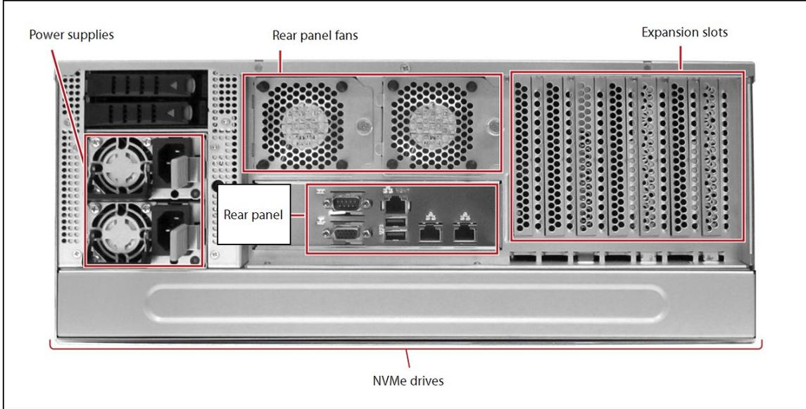
**Figure 12** The rear view of the Gen2 S Series BlackPearl 4U gateway.
