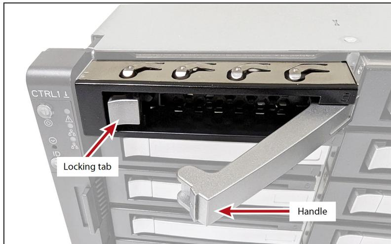
**Figure 297** Unlock the drive sled.
