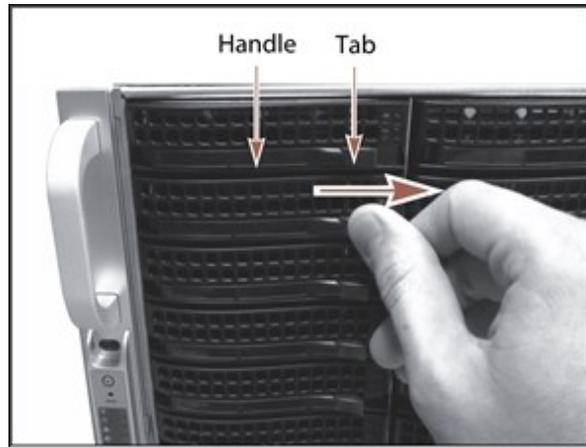
**Figure 321** Slide the tab to the right to release the drive sled handle.
