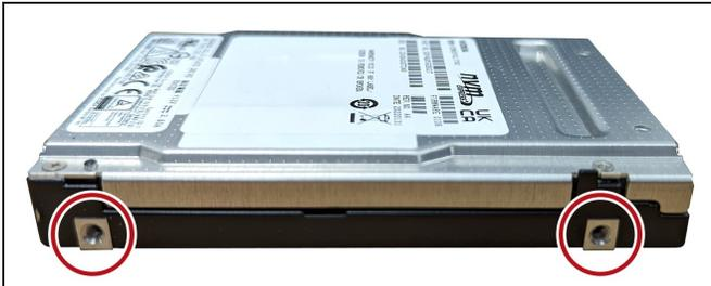
**Figure 308** Screw holes in drive.
