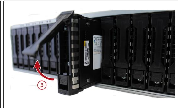
**Figure 320** Remove the drive sled with drive blank and insert the drive sled with drive.
