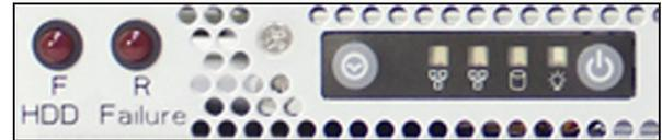
**Figure 174** The top left section of the front of the Gen2 V Series chassis, with the front bezel removed, showing system status LEDs.
