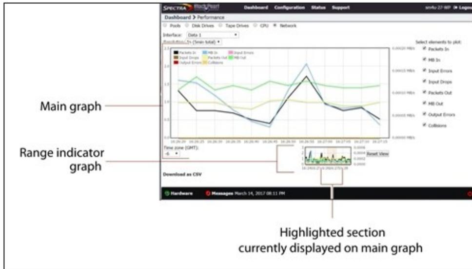
**Figure 193** Highlight a section of data to show in greater detail.
