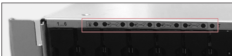
Figure 169 The top left section of the front of the Gen2 X chassis (front bezel removed) showing system status LEDs.
