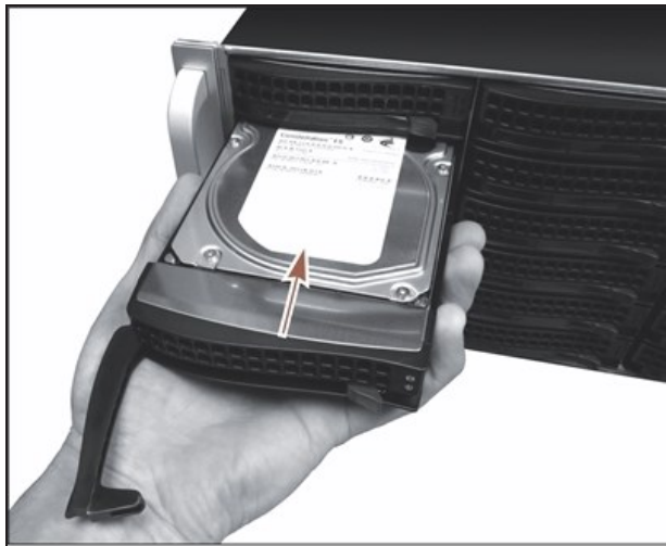
Figure 302 Install the drive into the BlackPearl gateway.
