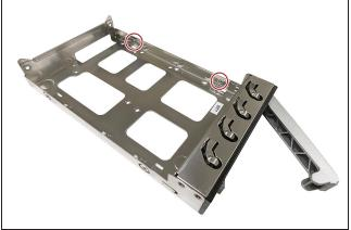
Figure 298 Screw holes in drive.
