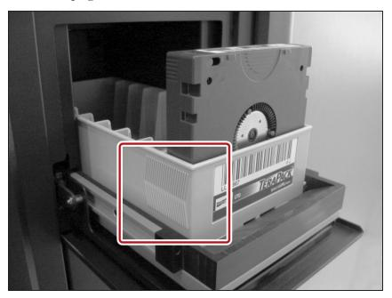
**Figure 263** Insert a magazine into the TAP, making sure that it is correctly oriented.
