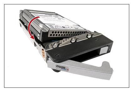
Figure 310 Install the drive into the sled.
