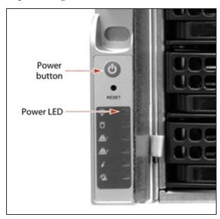
**Figure 27** Press the power button.
