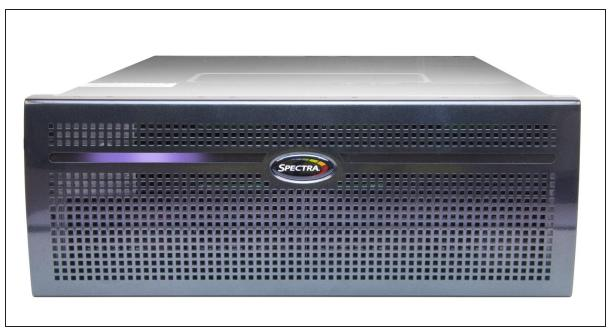
**Figure 1** A 4U BlackPearl chassis with front bezel and visual status beacon.
