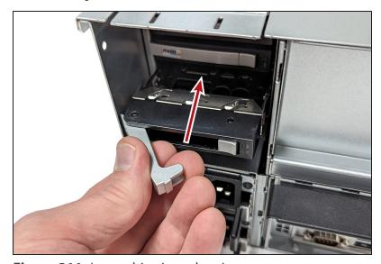
Figure 311 Insert drive into chassis.
