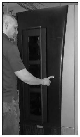
**Figure 284** Press the door release button to open the door.
