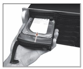
**Figure 323** Install the drive into the BlackPearl gateway.
