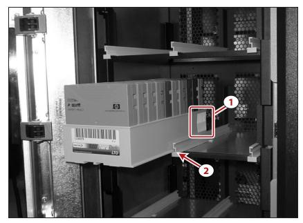
**Figure 258** Insert the magazine into the bulk TAP carousel, making sure that it is correctly positioned.
