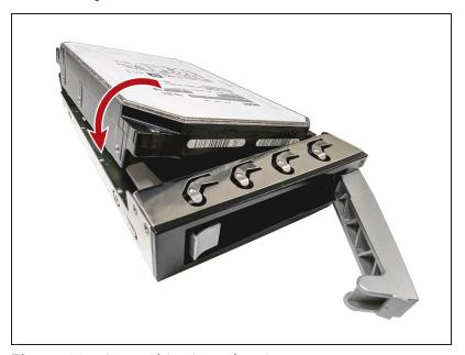
Figure 301 Insert drive into chassis.
