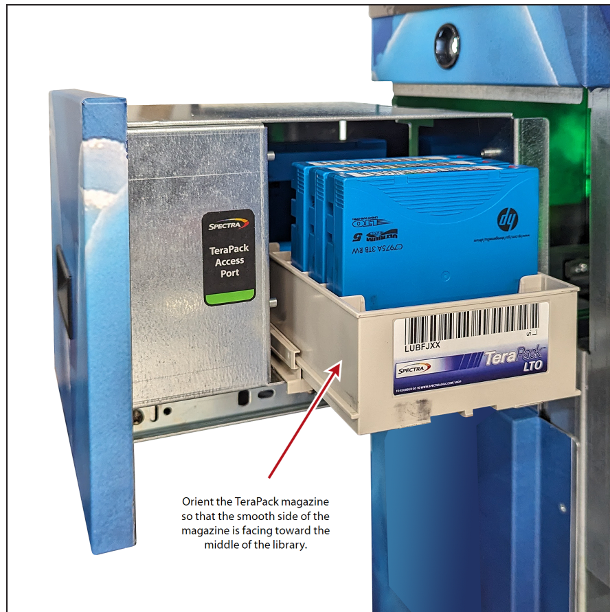
Figure 68 Insert a magazine into the TAP, making sure that it is correctly oriented.
