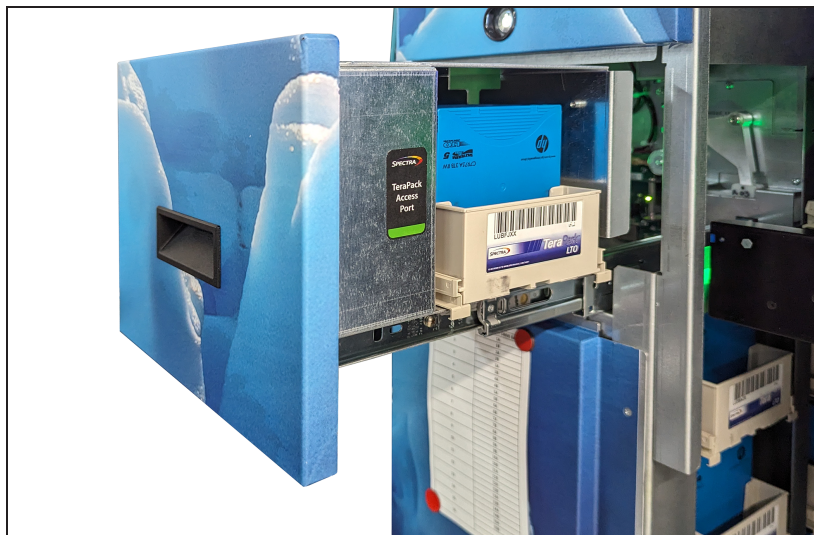
Figure 5 The TAP with a TeraPack magazine loaded.
