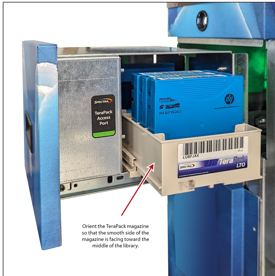
Figure 67 Insert a magazine into the TAP, making sure that it is correctly oriented.
