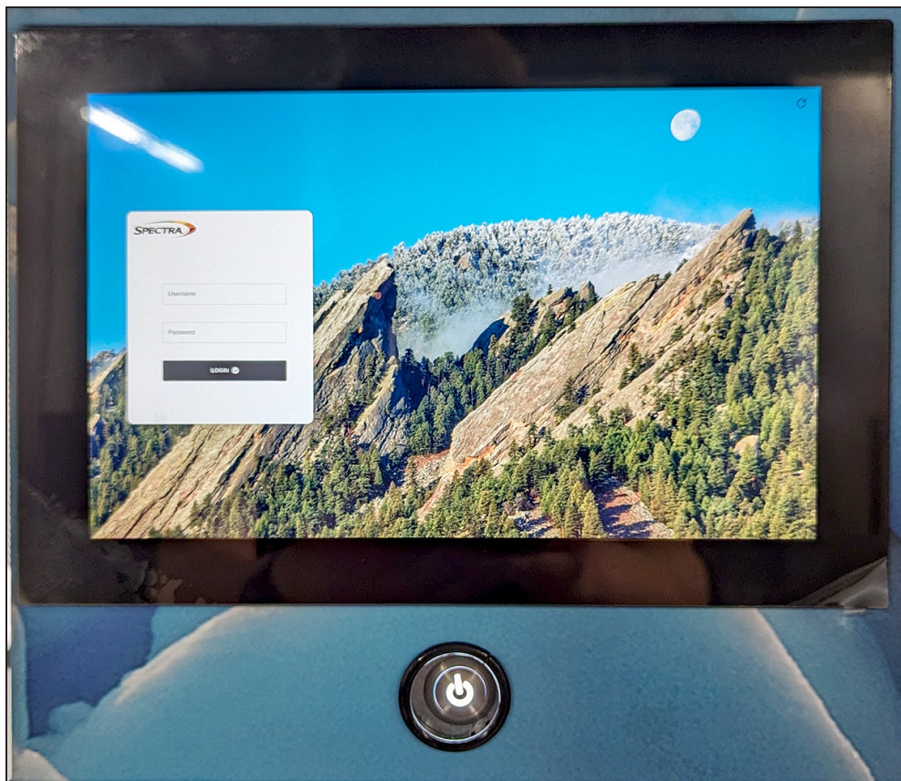
Figure 4 The library operator panel touch screen displaying the login screen of the LumOS user interface.
