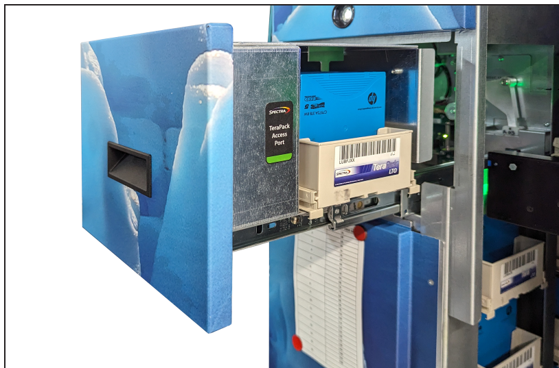
Figure 5 The TAP with a TeraPack magazine loaded.
