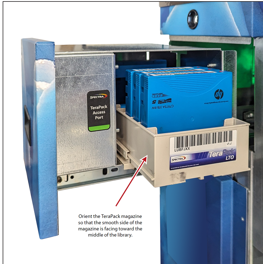
Figure 55 Insert a magazine into the TAP, making sure that it is correctly oriented.
