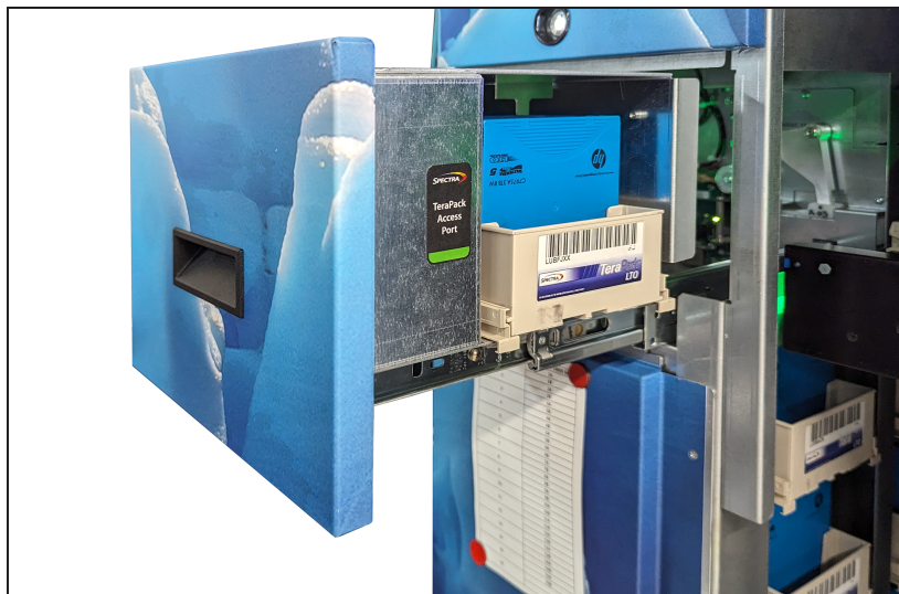
Figure 5 The TAP with a TeraPack magazine loaded.
