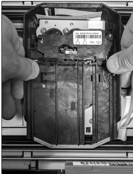
Figure 5 Grasp the robot as shown.
