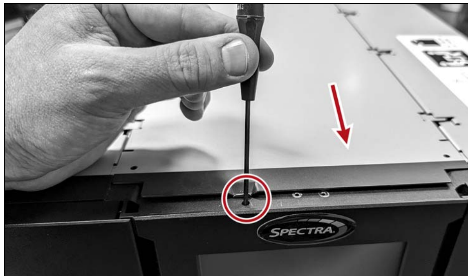
Figure 1 Release the cover latch.
