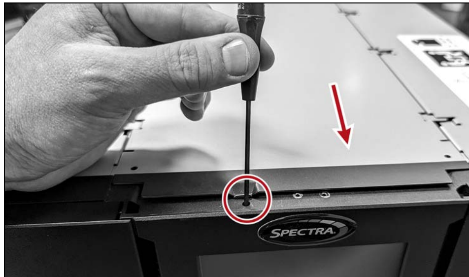
Figure 11 Release the cover latch.
