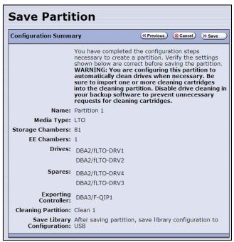
**Figure 126** The Save Partition screen for a storage partition that uses a Global Spare and a cleaning partition.
