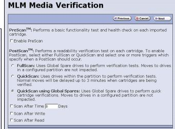
**Figure 116** The Media Verification screen when the partition uses LTO-5 and later generation drives.
