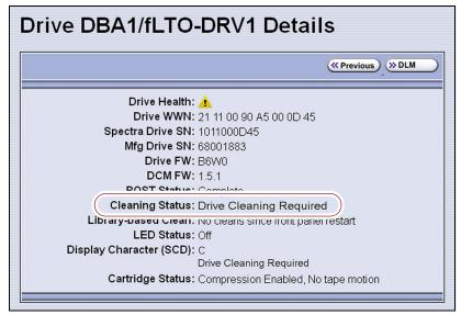
**Figure 295** The Drive Details screen, cleaning required.
