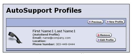
**Figure 192** Use the AutoSupport Profiles screen to manage profiles.
