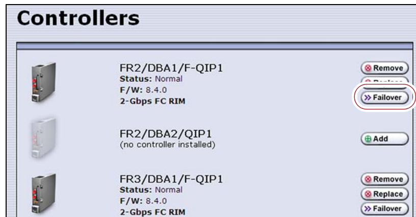
Figure 54 The Controllers screen before the failover controller is selected.
