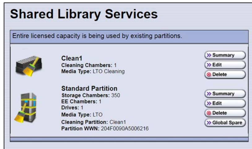
Figure 100 The Shared Library Services showing a cleaning partition and storage partition.
