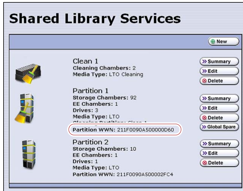
Figure 78 The WWN assigned to the partition.
