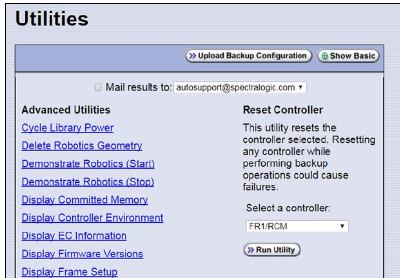
Figure 191 The Reset Controller utility for resetting a RIM.
