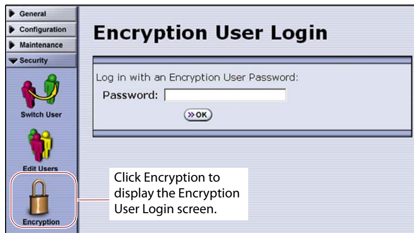
Figure 103 Log into the Encryption feature if you need to change the encryption setting for the partition.
