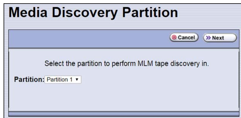
Figure 137 Select the partition containing the cartridges you want to add to the MLM database.
