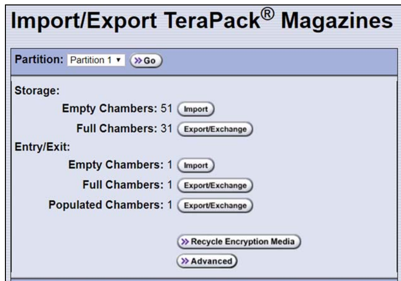
Figure 113 Use the Import/Export TeraPack Magazines screen to export or exchange magazines (storage partition shown).
