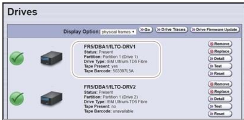
Figure 24 The Drives screen showing the component identifier for a drive.
