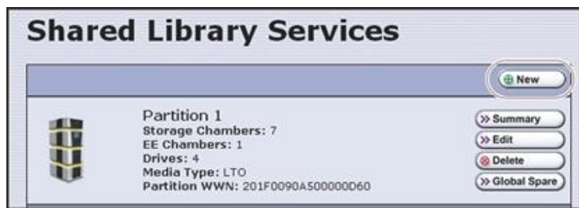
Figure 108 Click New on the Shared Library Services screen to begin creating the storage partition.
