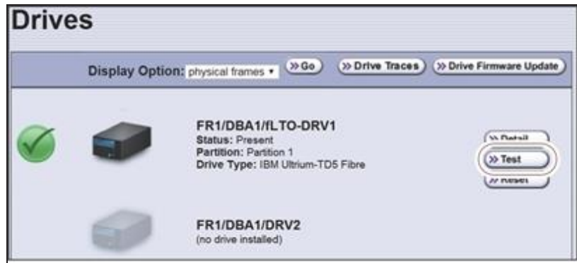
Figure 255 Click Test on the Drives screen to launch the wizard.
