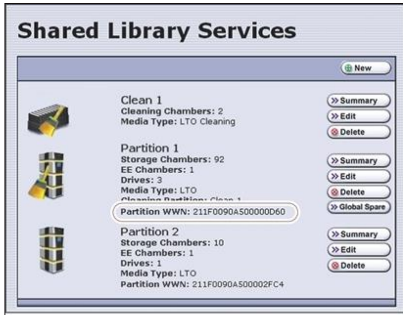
Figure 94 The WWN assigned to the partition.
