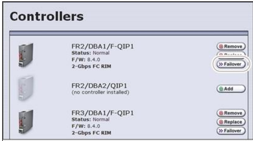
Figure 58 The Controllers screen before the failover controller is selected.
