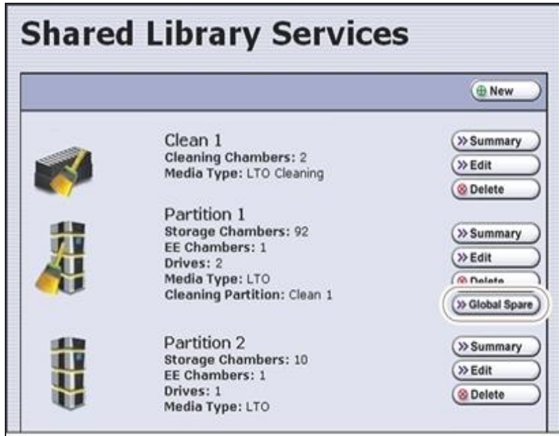
Figure 246 Click Global Spare to begin the process of replacing a partition drive with a Global Spare drive.
