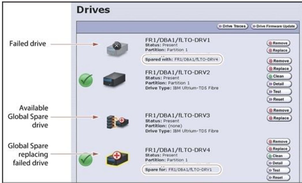
Figure 248 Check the Drives screen to confirm that the failed drive was replaced by a Global Spare drive.
