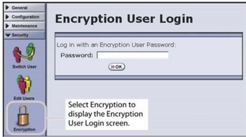
Figure 133 Log into the Encryption feature if you need to change the encryption setting for the partition.
