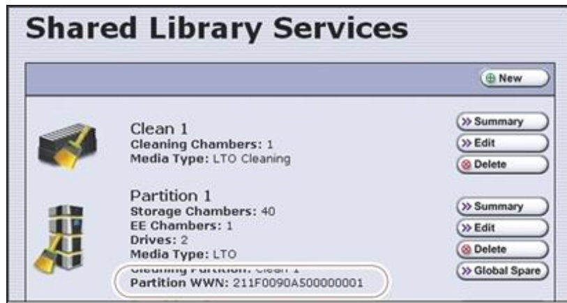
Figure 27 The WWN assigned to the partition.
