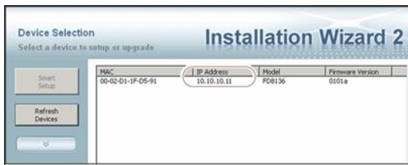
Figure 237 The camera IP address shown in the Network Camera Installation Wizard 2.
