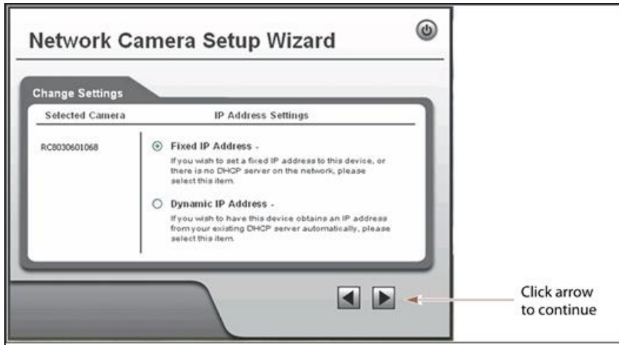
Figure 232 Select Fixed IP Address to configure the IP address for the camera.
