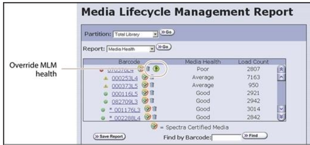
Figure 186 Click the green override button to reset the reported health for an MLM-enabled LTO cartridge.
