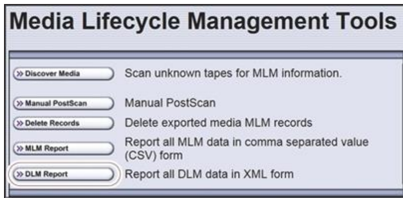
Figure 196 Click DLM Report on the Media Lifecycle Management Tools screen to export the DLM database as an XML file.
