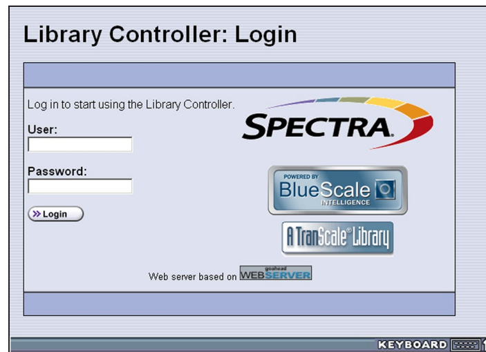
Figure 245 Log into the library using the Library Controller: Login screen.
