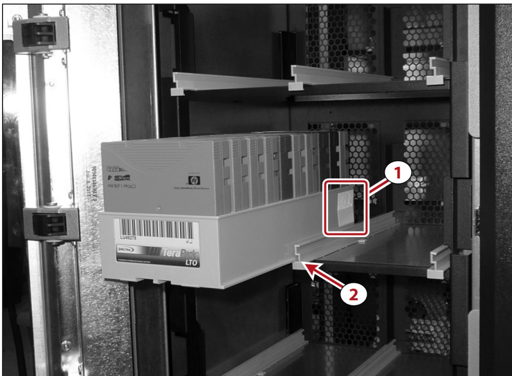
Figure 253 Insert the magazine into the bulk TAP carousel, making sure that it is correctly positioned.
