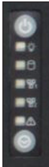
Figure 170 The top right section of the front of the Gen2 S Series chassis, with the front bezel removed, showing system status LEDs.
