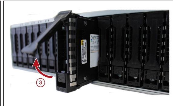
Figure 299 Remove the drive sled with drive blank and insert the drive sled with drive.
