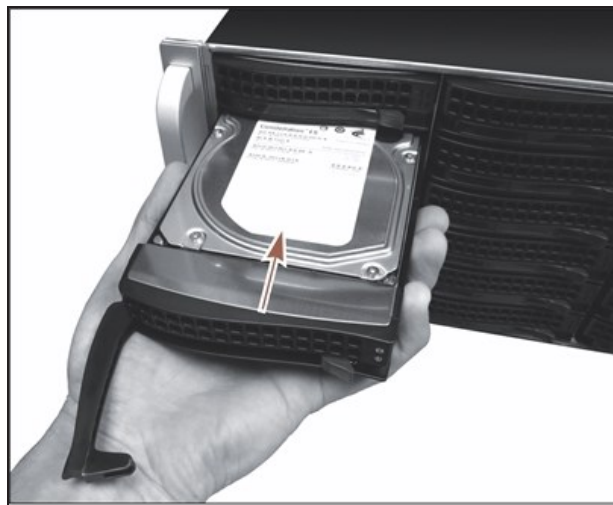
Figure 302 Install the drive into the BlackPearl gateway.
