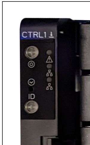
Figure 168 The Gen3 H Series chassis system status LEDs.
