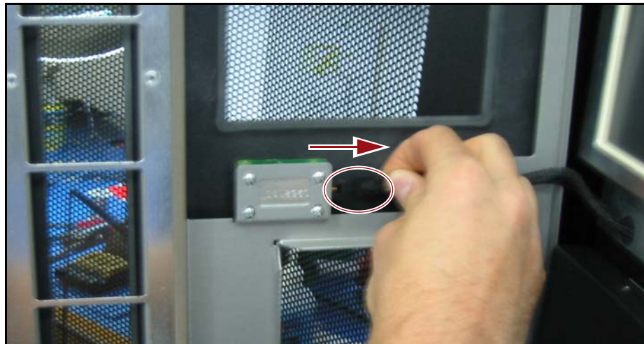
Figure 5 Disconnect the power switch cable.
