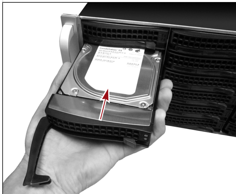
Figure 134 Install the drive into the Verde system.
